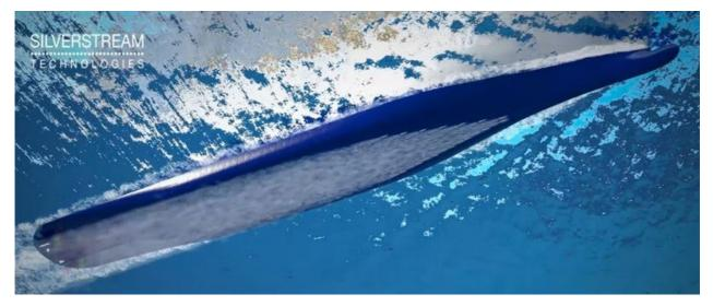
**Background:** Over the past decade, hull air lubrication has proven itself as a practical and scalable decarbonisation solution for the shipping industry. Air lubrication aims to reduce the frictional resistance of a ship, thereby cutting fuel burn and emissions.
