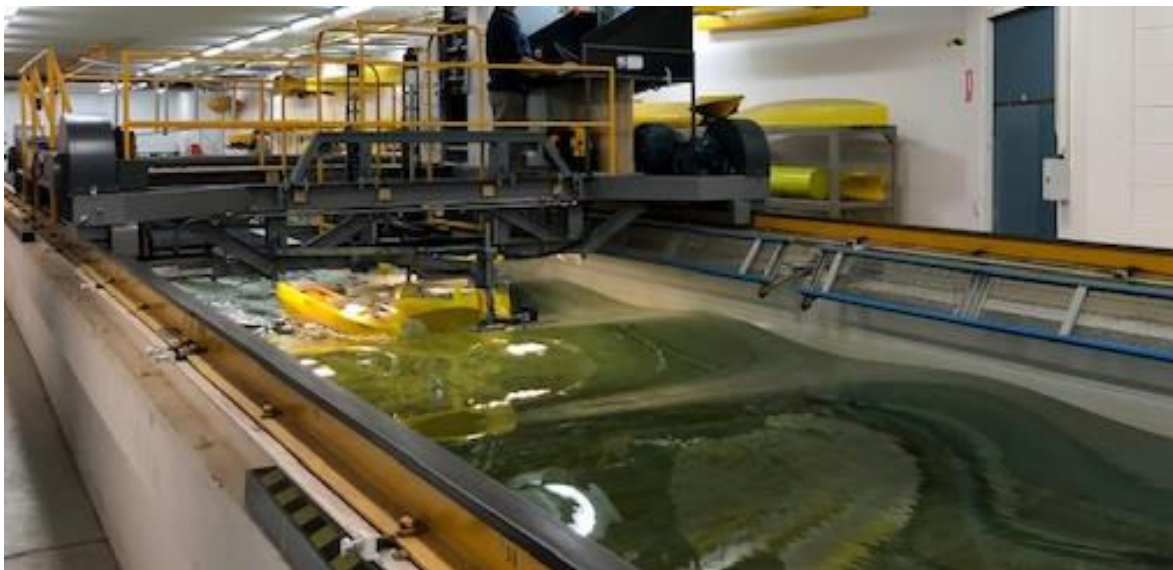
Figure 3: Showing the test model attached to the carriage of the towing tank facility at the Australian Maritime College, encountering a wave height of 72.7 mm at a speed of 1.53 m/s.
