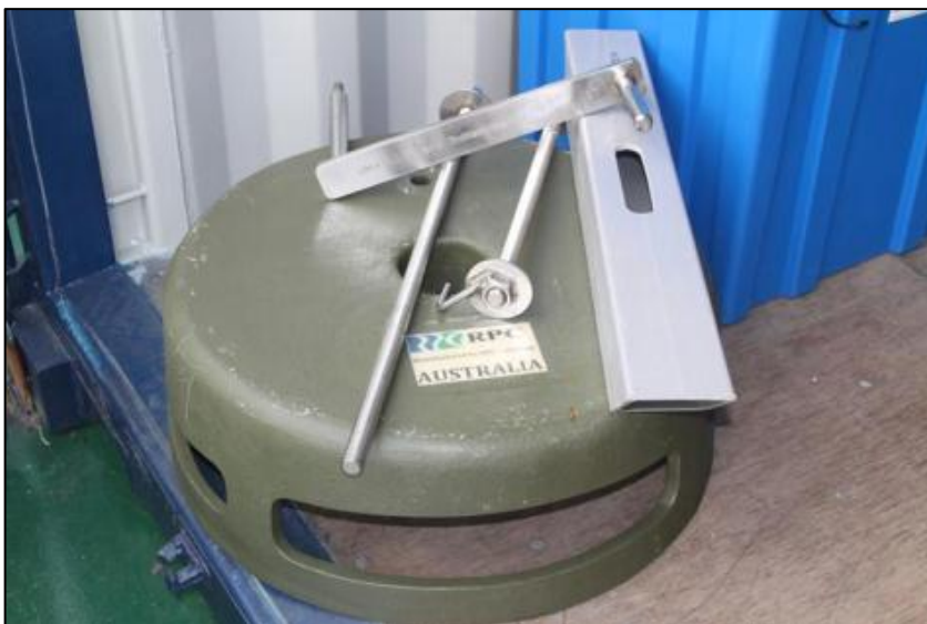
Figure 31 - The "Top Hat" Replacement Hatch Cover
