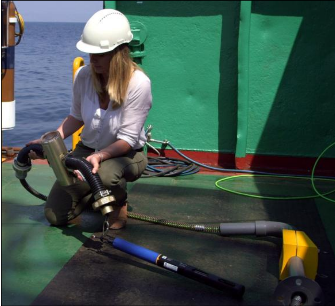
Figure 6 - Illustrating the manner in which the Data Umbilical was fed through to the Camera Module
