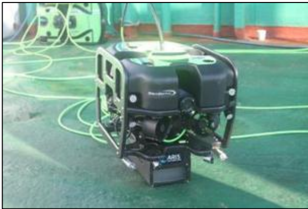
Figure 14 - The Modified vLBV with High Definition Camera & ARIS Sonar Deployed
