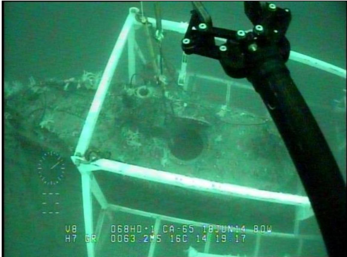
Figure 23 - Showing the Final Orientation of the Opened Upper Hatch
