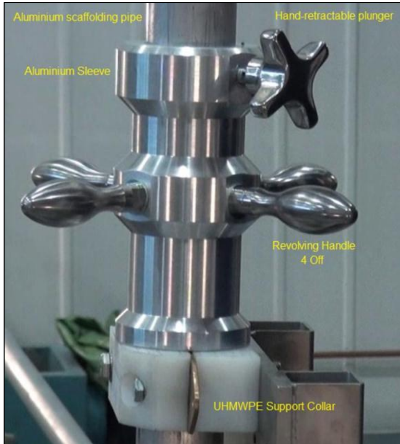
Figure 10 - Diver Operated Pole Cam Rotation System
