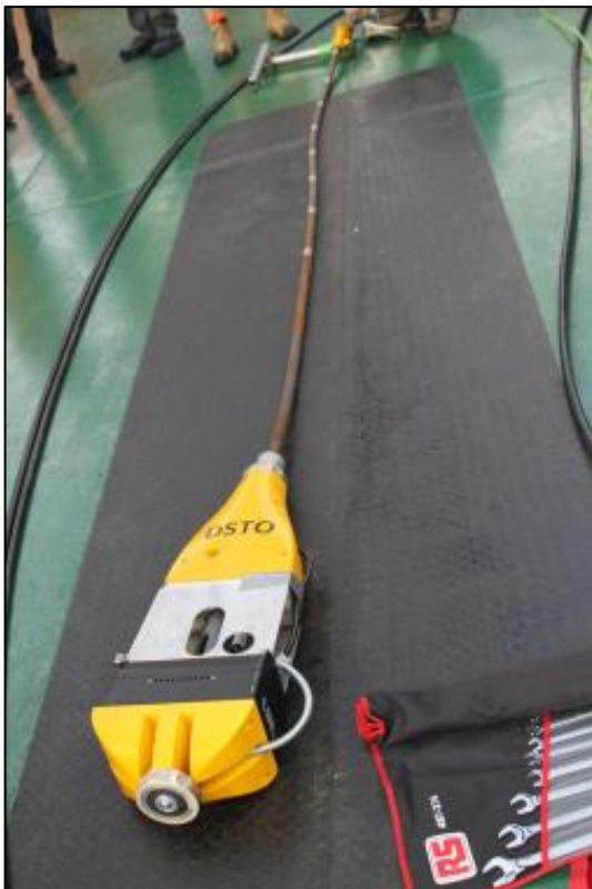
Figure 26 - The Modified "Pole Cam" which dispensed with the Pole
