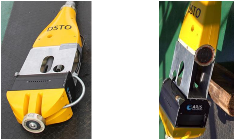
Figure 8 - Two Views of the Instrumentation Pod for the Pole Camera System
