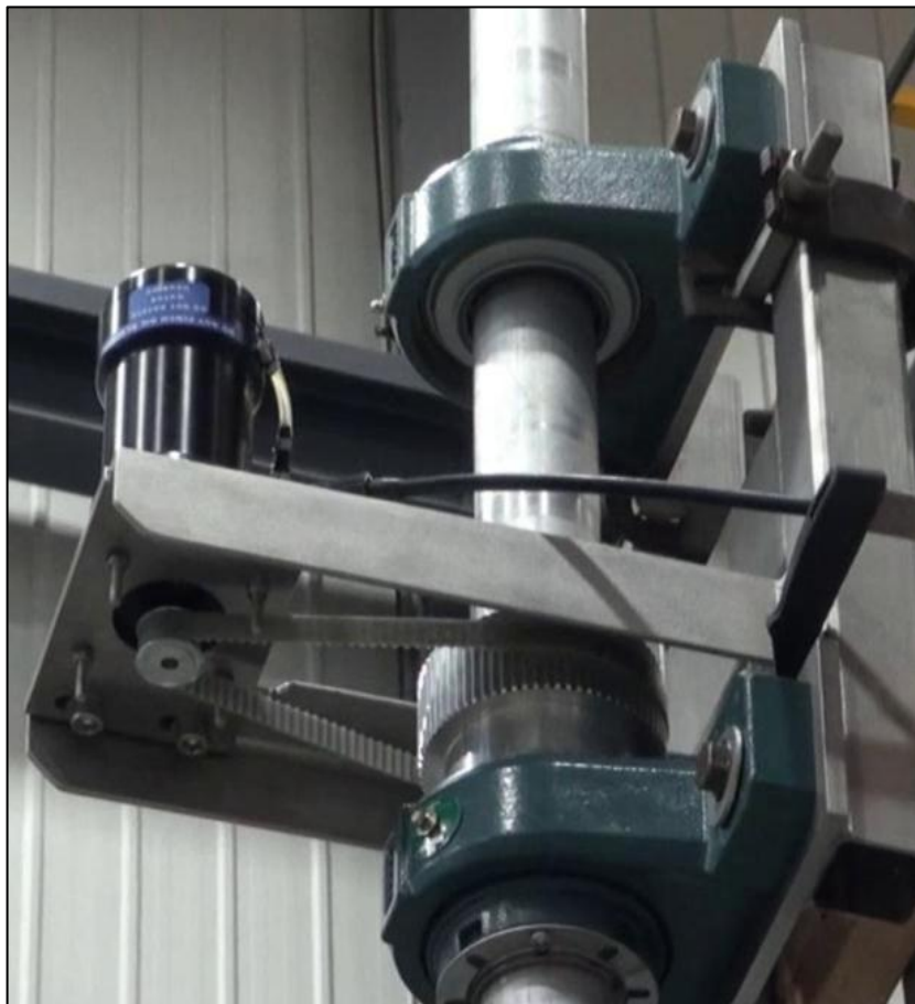
Figure 11 - Surface Controlled Pole Camera Rotation System
