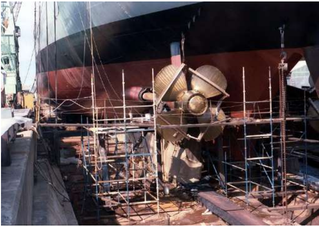
Temporary cleats were fitted to the CP Propellers prior to launching to prevent the blades changing pitch before the installation inboard was complete. The restricted space available at the entrance of No 1 Slipway prevented bilge keels being fitted for the launch.
