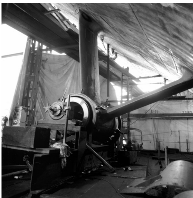
Shaft brackets and stern tubes were bored using portable boring machinery set up on the slipway (Image John Jeremy collection)
