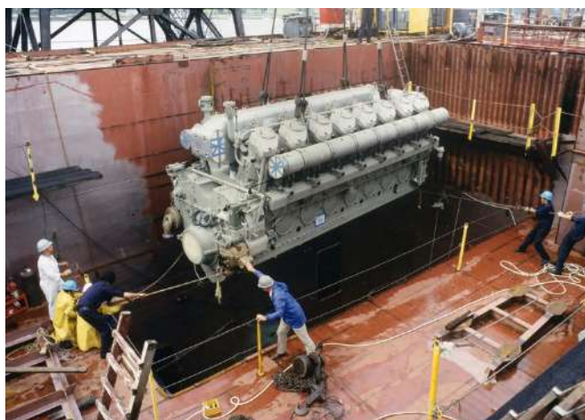
Lowering a main engine through a left-loose section of deck over the engine room
