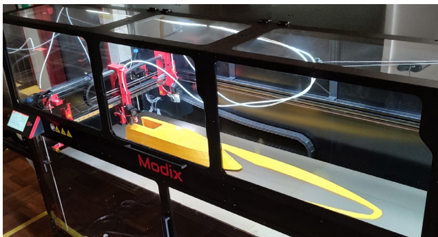
UNSW Canberra's Naval Architecture Group large-format ship hull Modix 180X 3D Printer displaying test prints of waterjet project hull form (Photo courtesy Sean McCracken)
