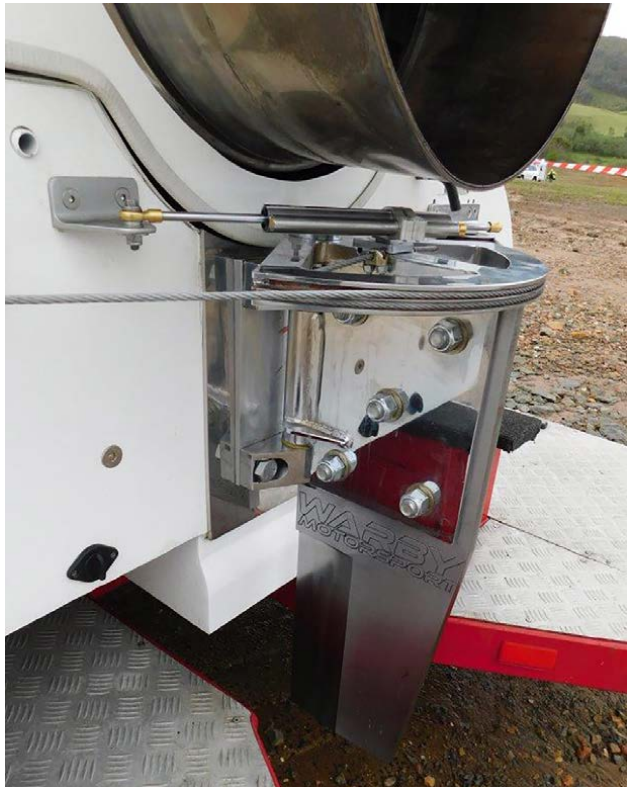
Rudder with damper fitted (Photo courtesy Martin Grimm)
