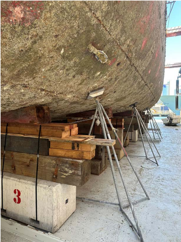
Tripod shores for sea lashing for the cold move (Photo courtesy Sean Langman)
