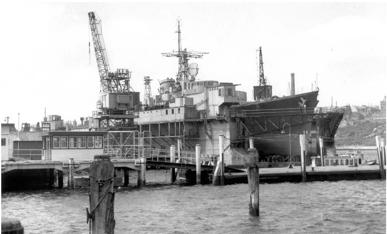
HMAS Queenborough in AFD17 at Cockatoo Island near the end of her conversion to a Type 15 anti-submarine frigate (Photo John Jeremy collection)
