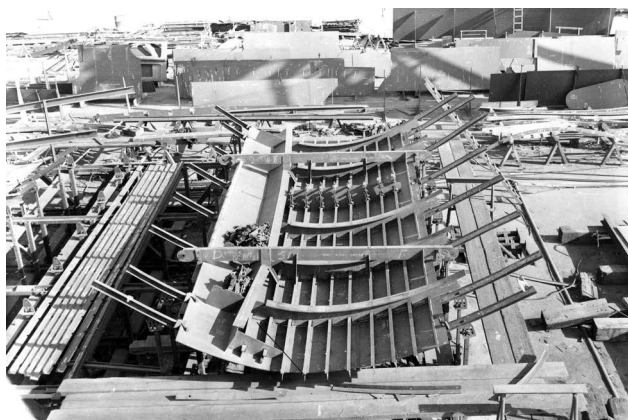
A shell panel for a Type 12 frigate showing the closely-spaced longitudinals (RAN photograph)
