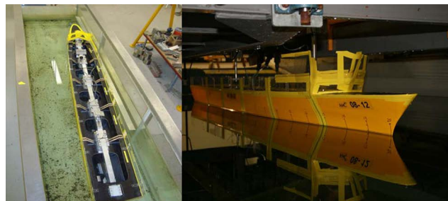
The numerical predictions were validated against published results obtained using a segmented model (Photos from Reference 1)
