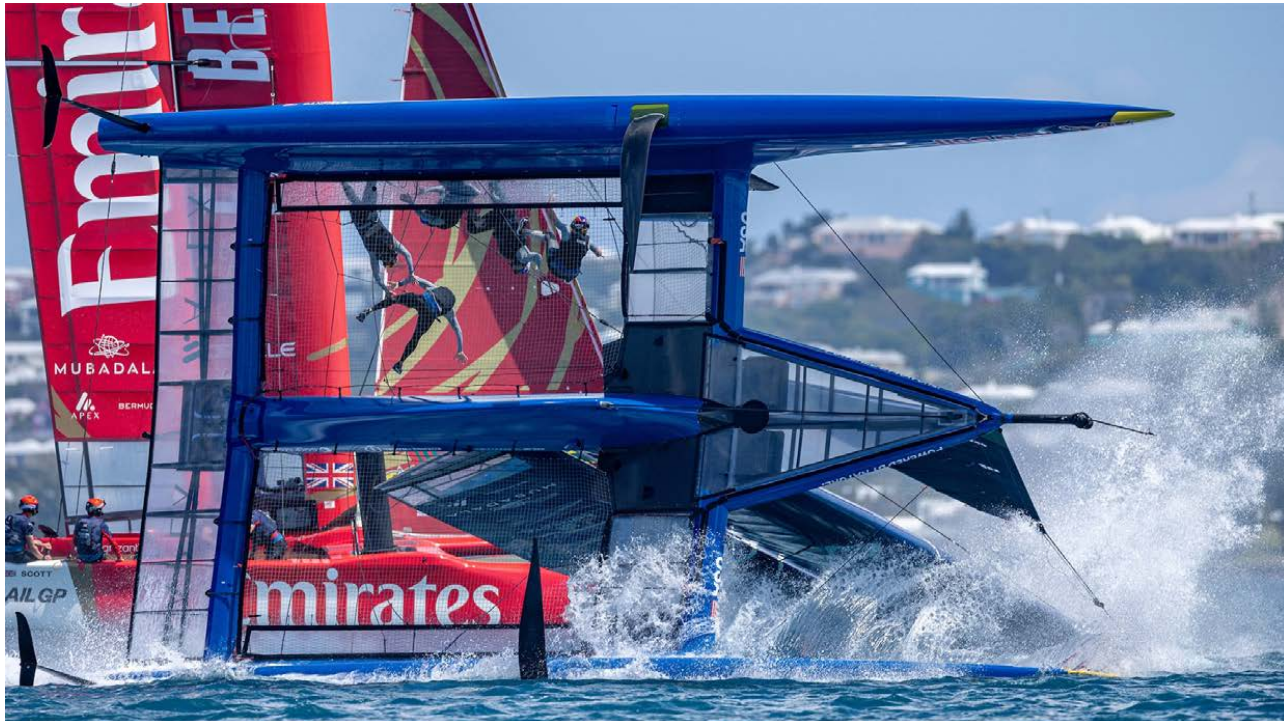
The United States' SailGP entry's dramatic pre-racing capsizes during the third fleet race of the practice day in Bermuda when the US team was on the reach to Mark 1. The top of the wing inverted—or bent the wrong way—resulting in the F50 suddenly flipping over and five of six crew-members falling overboard (Photo courtesy SailGP)
