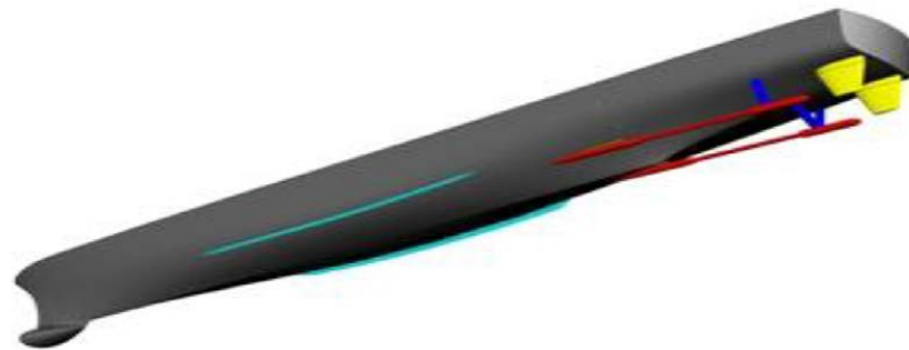
Figure 1: The DTMB 5415 hullform is shown with highlighted appendages. Bilge keels are marked in teal, drive shafts in red and rudders in yellow [11]
