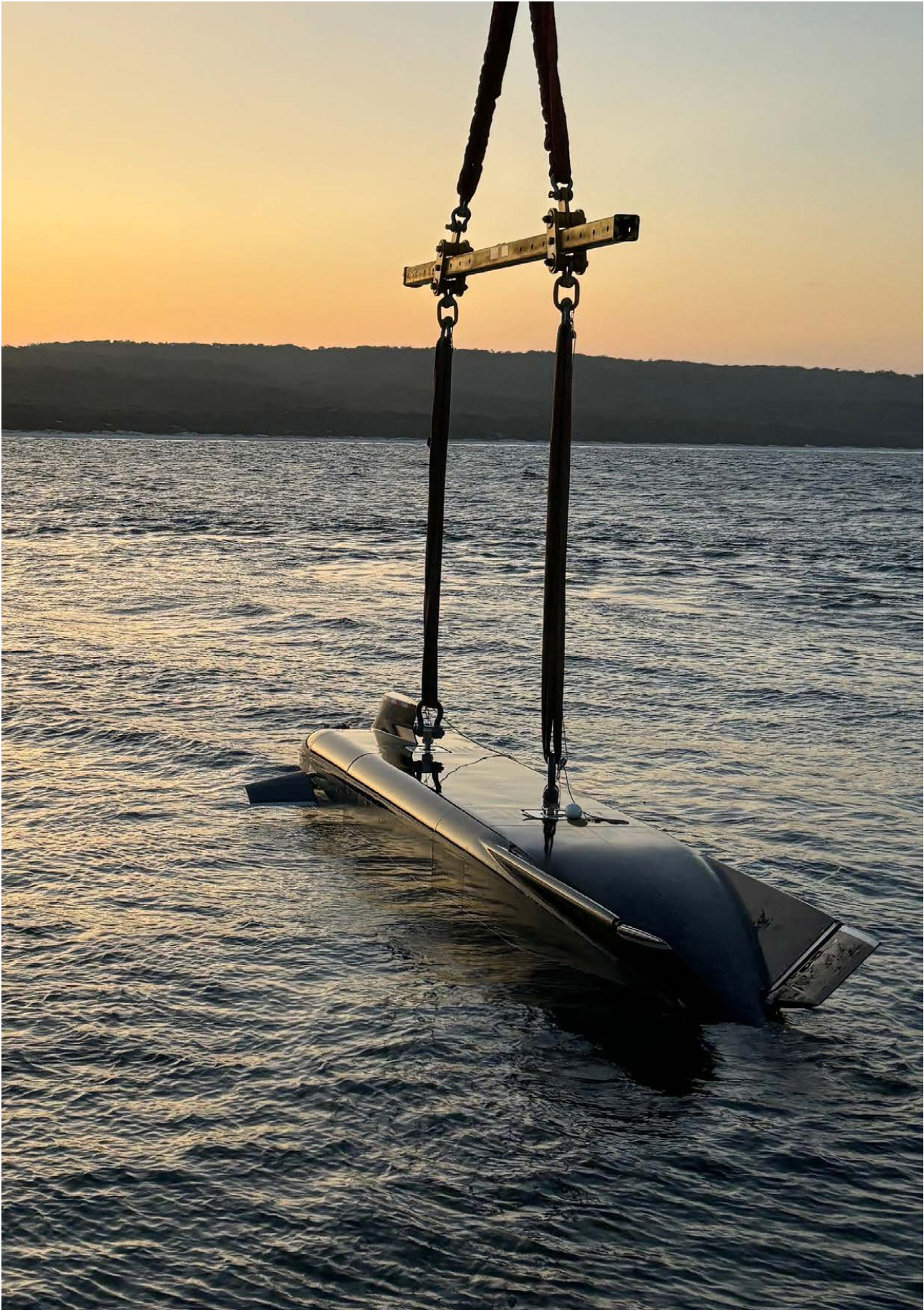
Australia's first developed extra large autonomous undersea vehicle (XLAUV), Ghost Shark , is being jointly developed and funded by a partnership between Defence and Anduril Australia, and will provide the Navy with a stealthy, long-range autonomous undersea warfare capability (RAN photograph)
