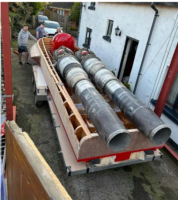
Cockpit mould and jet outlets on Longbow (Photo from Longbow website)
