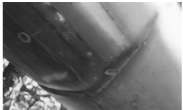
A close up photo of the transverse step and associated air feed pipes (two of three visible) incorporated in the hull of ZAP . The hole well aft of the step is for a rudder stock. (Photos courtesy Martin Grimm)
