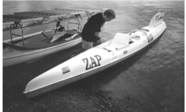
Dale Siver attends to ZAP . Its air feed step is positioned below and slightly forward of the front of the 'cockpit' area.
