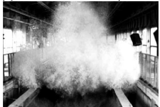
A giant wave produced with a hydraulically-powered wave generator in the Giant Wave Tank in Hanover in 2002. (Photo Technical University of Berlin)
