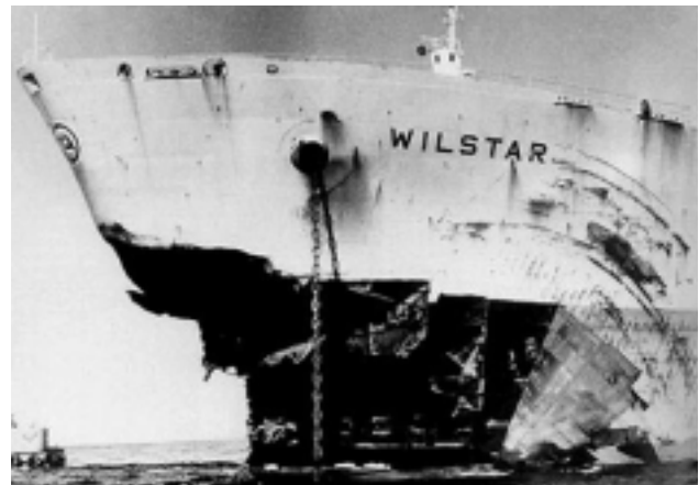
Rogue waves are most common in the Agulhas current off the east coast of South Africa, with numerous well-documented cases of extreme individual waves, including some striking photographs of damaged ships. This bow damage was received by Norwegian tanker Wilstar in 1974. (Photo DLR)
