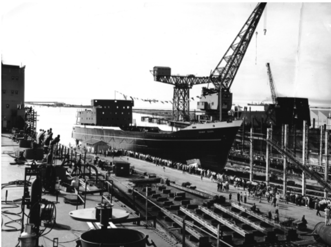
The above photograph shows the launching at Whyalla of the Union Steamship Company's Seaway Queen on 19 November 1963. The 107.89 m LBP roll-on/roll-off ferry was of hybrid design with lift-on/lift-off cargo facilities as well. Completed in 1964, she served with the Union Company until 1980. In the background her identical sister Seaway King is under construction. She was launched 8 weeks later. The 21 600 t dwt bulk carrier Gerringong is in the left foreground. (Photo Bryan Chapman collection)
