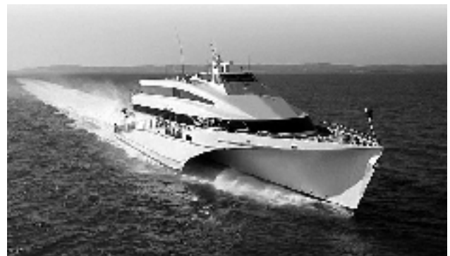
Figure 11: MV Triumphant at 40 knots — note the effectiveness of the bow spray chine in keeping the vessel dry.
