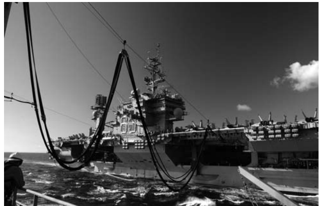
With the ships connected by highwires, two cargo fuel hoses from Success approach Kitty Hawk . A probe on the end of each hose connects with a fitting on the receiving ship allowing fuel to pass (RAN Photograph)
