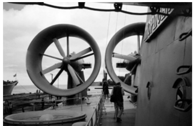
View on deck of Zubr showing one (of four) lift fans and two (of three) propulsion fans (Photo courtesy Lawry Doctors)
