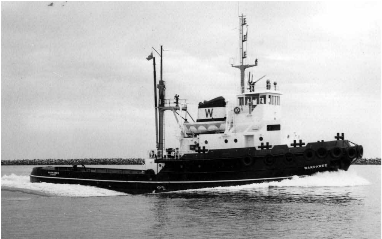
The tug Warrawee , Adelaide Ship Construction Ship No. 55, was completed in 1970 for Adelaide Steamship Industries Pty Limited. The 40.9 m tug had a bollard pull of 60 t and was designed by Burness Corlett and Partners (Photo John Jeremy Collection)
