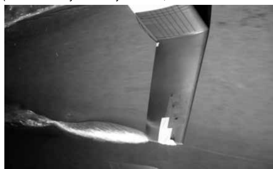
Figure 5 — The T-Foil being tested in the towing tank. The stick on hot-film probes can be seen just inboard of the tip of the ventilating foil. Complete foil ventilation follows shortly afterwards.
