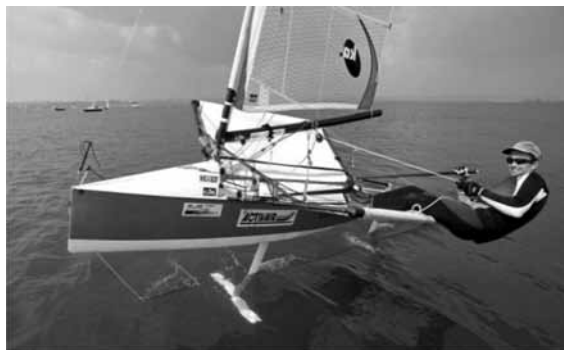
Figure 4 — A Moth dinghy on hydrofoils. The centerboard and rudder T-Foils can be seen beneath the water surface. (Photo courtesy of Thierry Martinez, © www.thmartinez.com)
