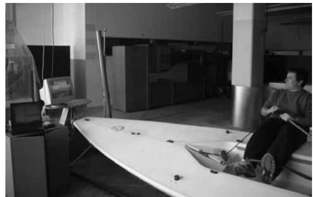
Figure 7 — Robert Maher sailing the VSail-Researcher against his Matlab simulation running on the laptop in the left of the picture.
