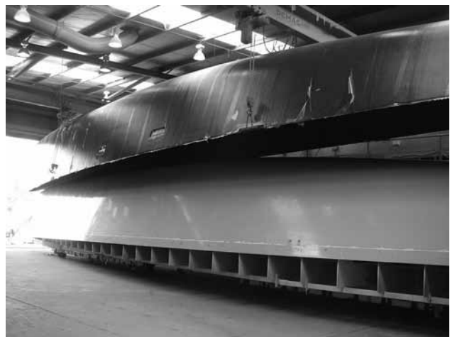
Singularity 's hull being lifted off the mould at McConaghy Boats (Photo courtesy McConaghy Boats)
