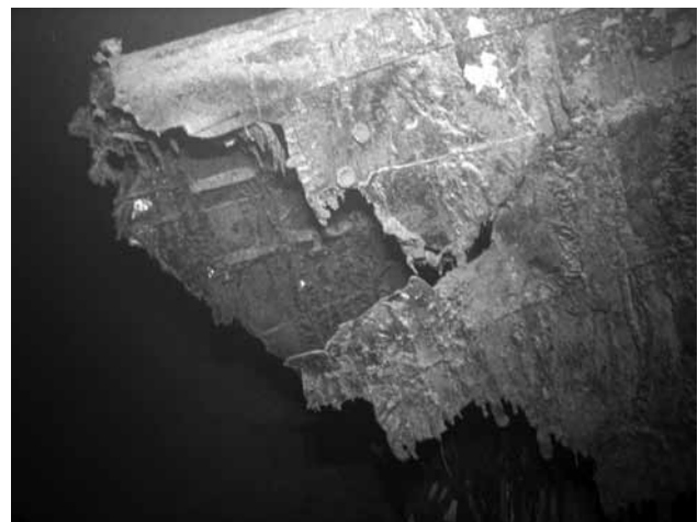
The aft end of the upturned bow section of HMAS Sydney showing the indentation of the shell plating caused by the torpedo hit (Finding Sydney Foundation photo by David Mearns)
