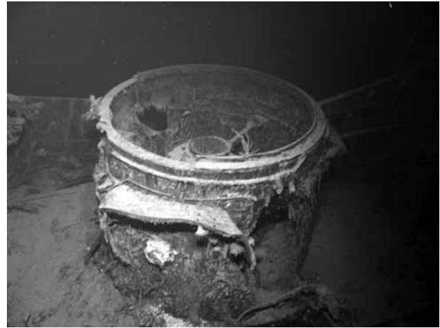
The base for the director control tower on HMAS Sydney showing hits on the port and starboard sides by 15 cm shells from Kormoran (Finding Sydney Foundation photo by David Mearns)
