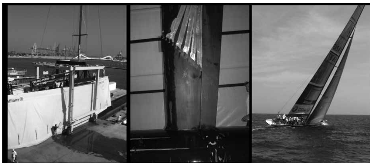
Figure 3 — Experimental set-up using the hot-film probes for full scale work in 2006. Stick-on hot-film probes shown in-situ on the keel in the centre image.
