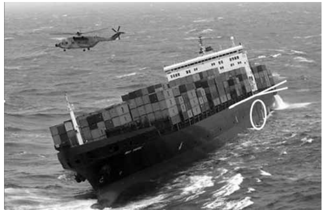
MSC Napoli on 18 January 2007 (note vertical dark line indicating compression buckling below, and change of deck line at, forward end of superstructure) (Photo courtesy DNV)
