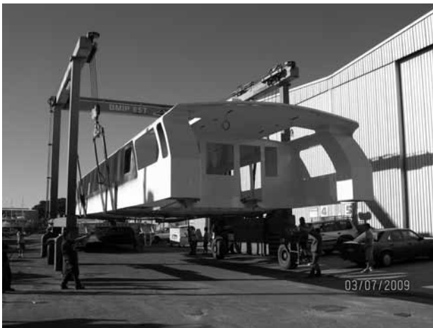
Painted composite superstructure ready to be bonded to the aluminium hull (Photo courtesy SSM Boatbuilding)
