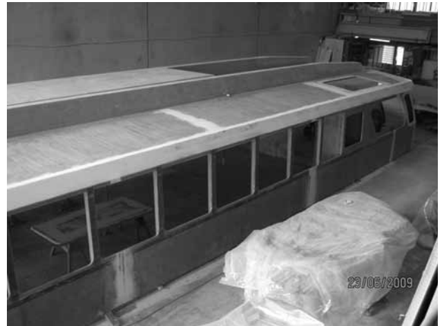
Assembly and fairing of the composite superstructure (Photo courtesy SSM Boatbuilding)
