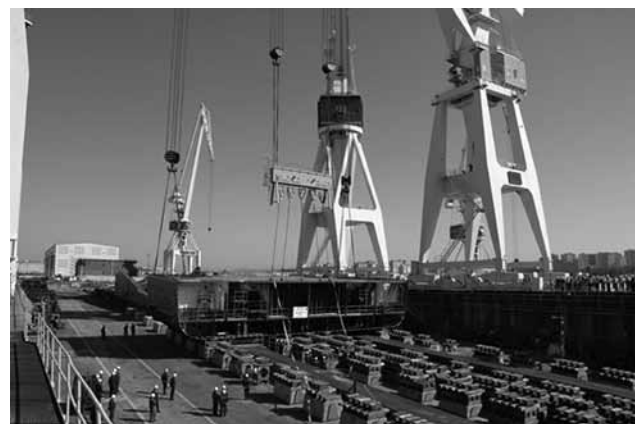
The first module for LHD 01 being placed on the slipway at Ferrol in Spain (Photo courtesy Navantia)
