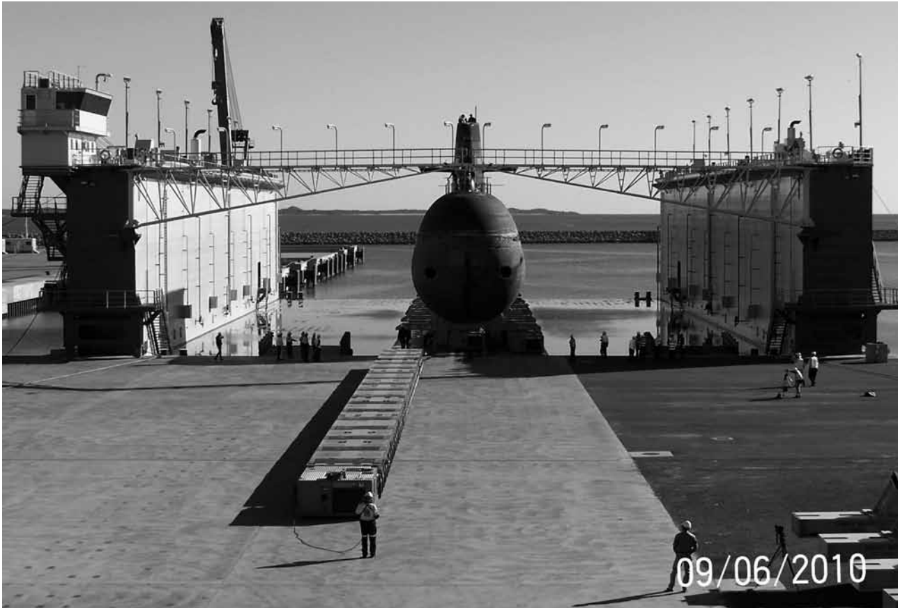
HMAS Farncomb in the floating dock with the two pairs of rams anchoring the dock to the wharf, two SPMTs threaded under the cradle and the third one being inserted. The SPMT operator is in the foreground and part of the second submarine cradle in the lower right corner (Photo courtesy Hugh Hyland)
