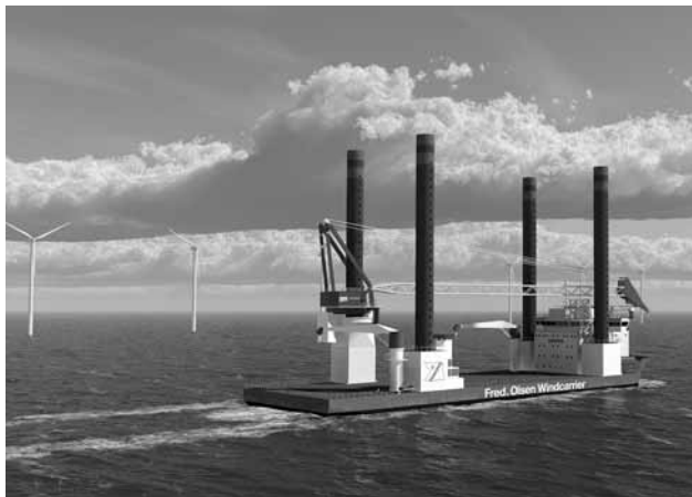
The new wind turbine installation vessel owned by Fred. Olsen Windcarrier AS, will be powered by an integrated Wärtsilä ship power system.
