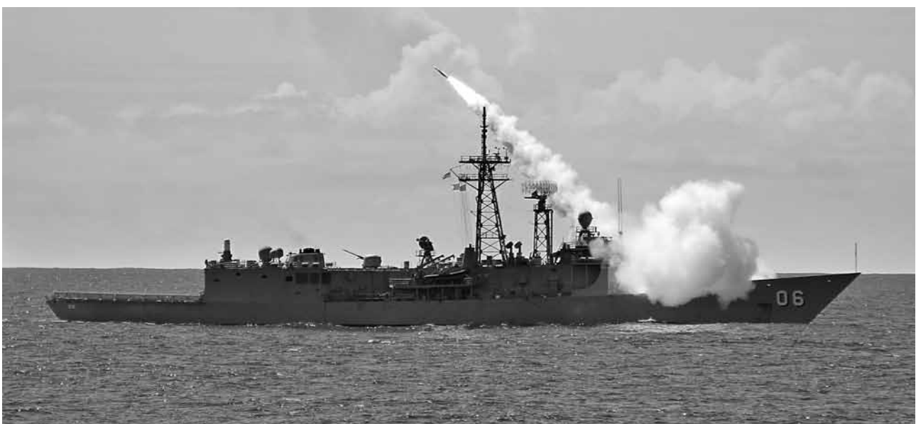
HMAS Newcastle firing a Standard Missile (SM-2) as part of a surface-to-air missile exercise with HMAS Warramunga during RIMPAC 2010. The exercise was conducted on the Pacific Missile Range Facility to test the operation of integrated multi-ship defence against multiple targets with SM-2, Evolved Sea Sparrow Missile (ESSM), Nulka and Chaff. Realistic targets (BQM-74E) representing a regional subsonic ASM were used. (RAN photograph)
