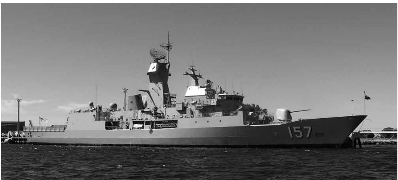
A recent photograph of the Anzac-class frigate HMAS Perth after the anti-ship missile defence upgrade. The new mast carries the CEA phased-array radar and the quarter deck has been enclosed (Photo courtesy Hugh Hyland)
