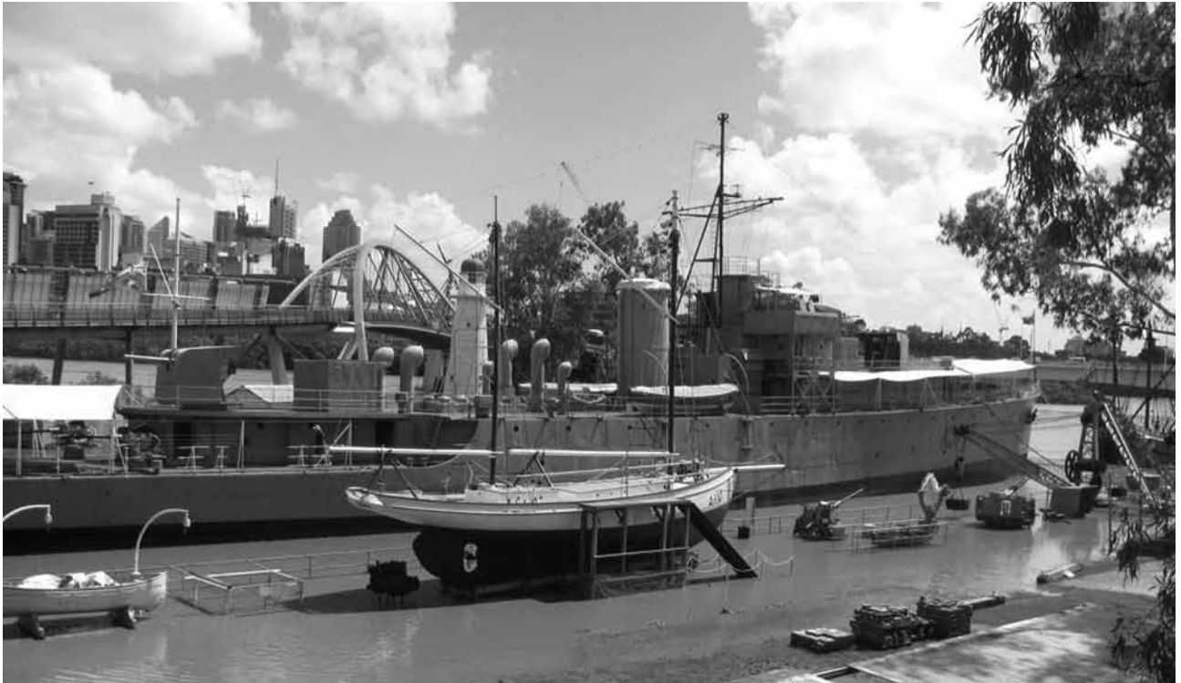
The recent brisbane floods refloated the WWII frigate Diamantina in the South Brisbane graving dock at the Queensland Maritime Museum. Diamantina floated up satisfactorily, but the lightship CSL2 (astern of Diamantina , was not so lucky. With some plating missing from her hull, CSL 2 began to float but then sank in the dock (Photo courtesy Brett Smith)
