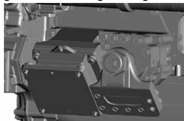
Integrated engine carrier and shock limiter (Image courtesy MTU)
