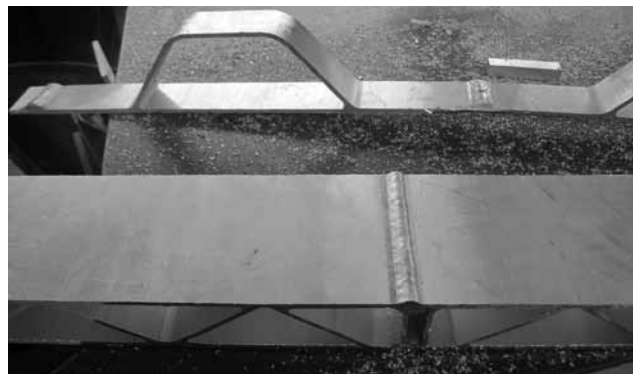
Aluminium sections used for passenger decks (top) and vehicle decks (Photo Phil Helmore)
