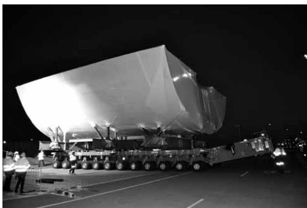
The first air-warfare destroyer (AWD) block to be shipped by sea from interstate arrived at the Government of South Australia's Common User Facility wharf on 15 August. AWD block 109, built by BAE Systems at Williamstown, was successfully rolled off the barge and into ASC's AWD shipyard where it will be housed until the consolidation process begins in 2012 (Photo Department of Defence)
