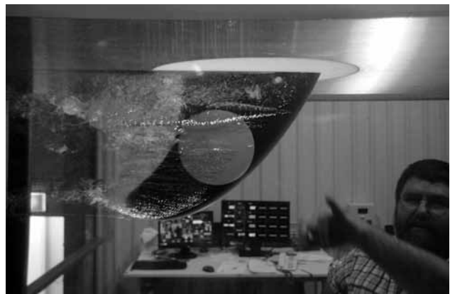
Bryce Pearce explaining details of cavitation on a surfboard fin (Photo Phil Helmore)
