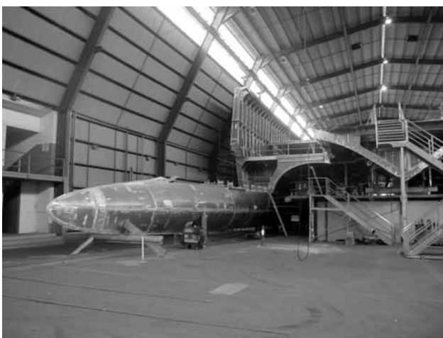
Wave-piercing bow on the 99 m vessel (Photo Phil Helmore)
