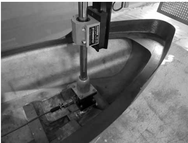
Bluefin model, showing the forward towing post and the load cell (Photo Phil Helmore)
