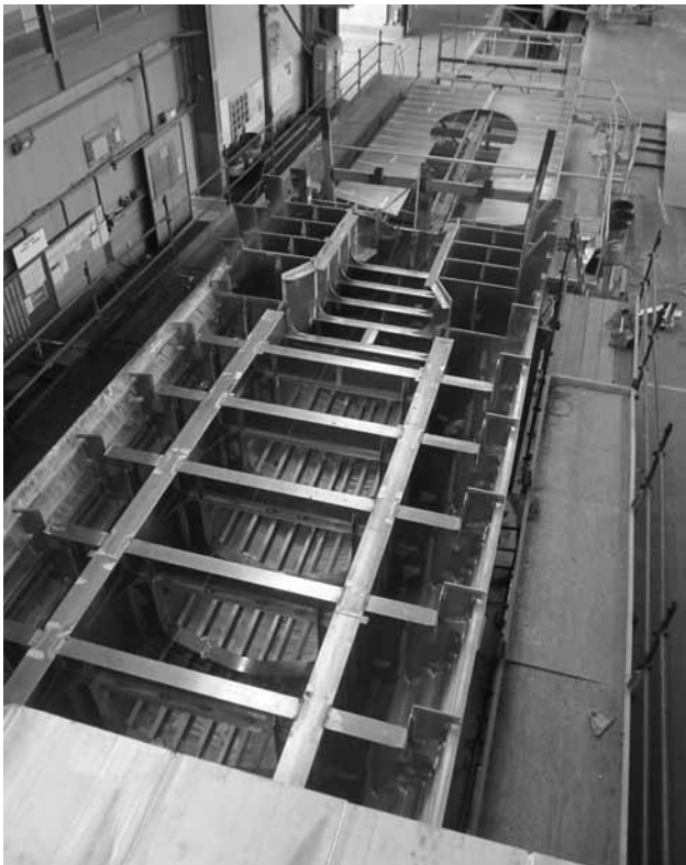
Engine beds, gearbox foundations and cut-out for waterjet intake on the 99 m vessel (Photo Phil Helmore)
