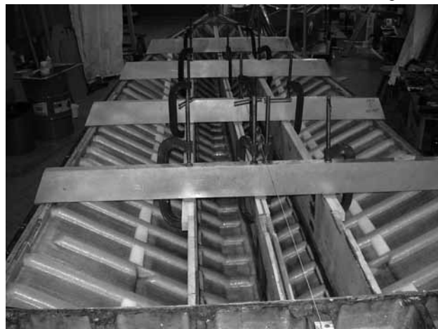
Figure 1 — Example of internal structure of single skin hull bottom
