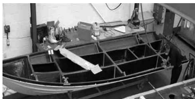
Figure 2 — Example of internal structure of sandwich hull bottom
