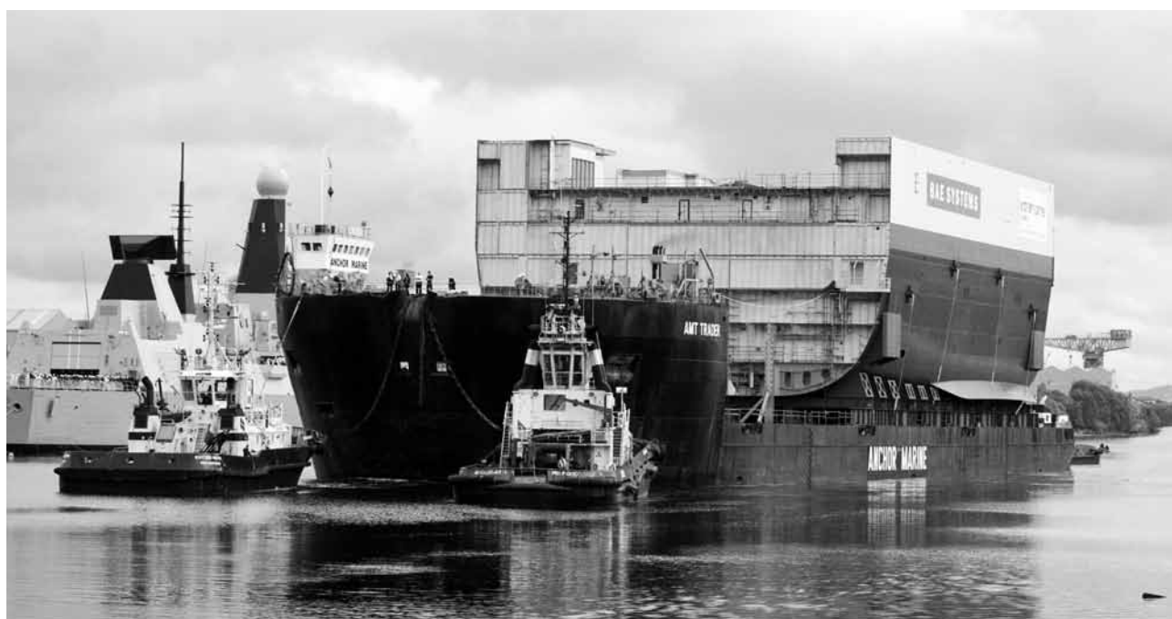
Lower block 03 for the Royal Navy's new aircraft carrier HMS Queen Elizabeth leaving the Clyde recently for Rosyth where the ship will be assembled. The size of the 8000 t block can be gauged by the Type 45 destroyer in the background (Photo courtesy BAE Systems)
