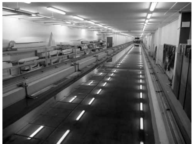
The AMC towing tank, showing some of the models and the beaches (Photo Phil Helmore)
