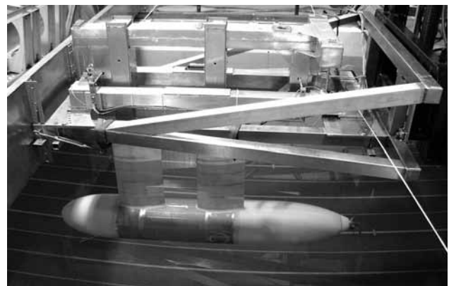
Figure 7: The large 6-DOF force balance mounted on a steel frame which is attached to the hydraulic lifting equipment.
