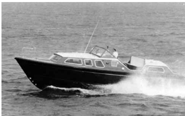
This 12.1 m Admiral's Barge was built of cold-moulded wood and was delivered to the RAN in 1992 (Photo Norman R Wright & Sons Archives)
