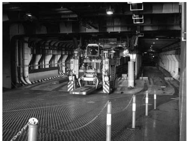
A straddle carrier handling a steel slab in Iron Monarch (Photo courtesy Teekay Shipping Australia)
