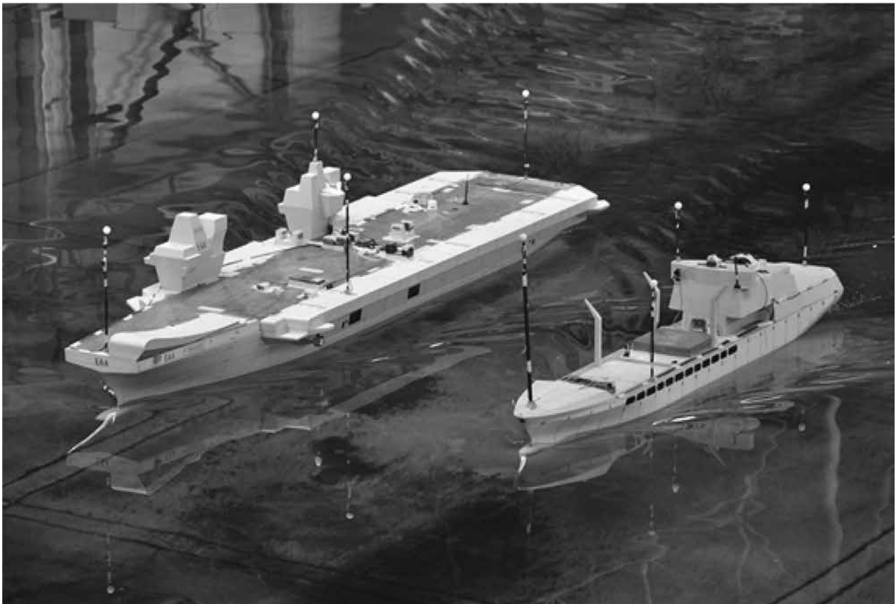
The models of HMS Queen Elizabeth and RFA Tidespring in the tank at Haslar (QinetiQ photograph)
