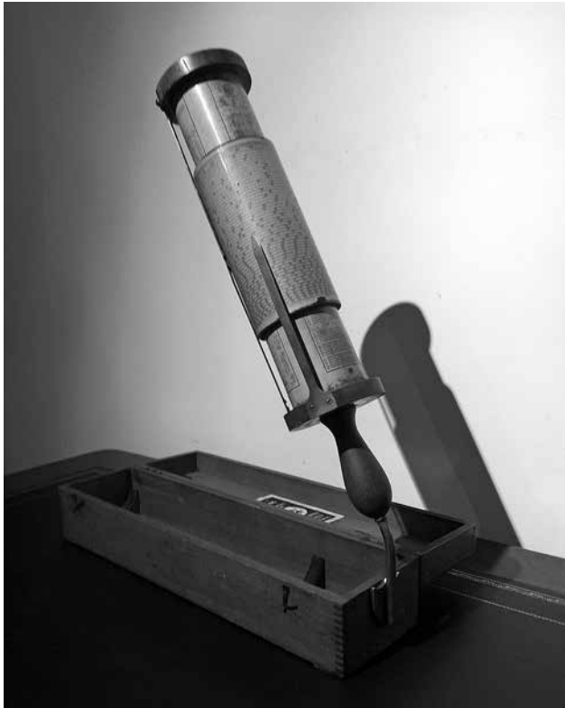
The cylindrical Fuller Calculator, made in England by Stanley, was first produced in the nineteenth century and was equivalent to a slide rule 12.4 m long. It is said that a skilled operator could produce accurate results to six decimal places (Photo John Jeremy)
