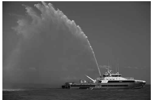
Amanah 1 testing her fire monitor (Photo courtesy Incat Crowther)
