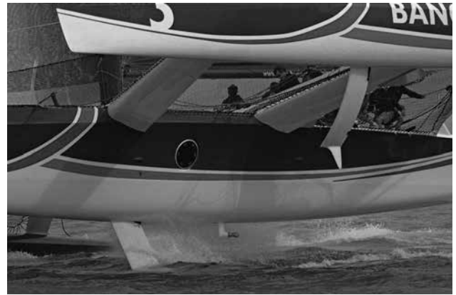
Team Australia (as Banque Populaire) showing the curved lift foils (Photo courtesy Sean Langman)
