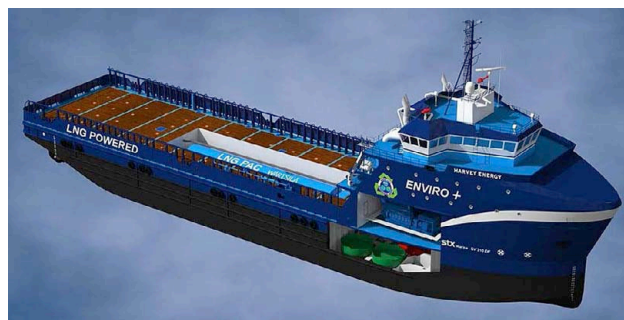
Cutaway view of Harvey Energy showing the LNGPac fuel system by Wärtsilä (Image from HHPInsight website)
