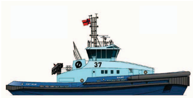
The new escort tugs contracted by Østensjø Rederi will feature a Wärtsilä solution including dual-fuel engines integrated with a customised gas storage and supply system (Image courtesy Robert Allan Ltd)
