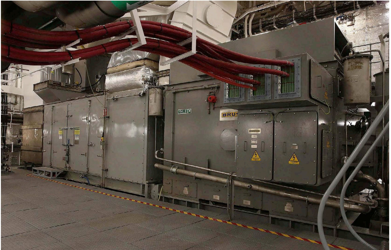
The gas turbine alternator on board HMAS Canberra (RAN photograph)
