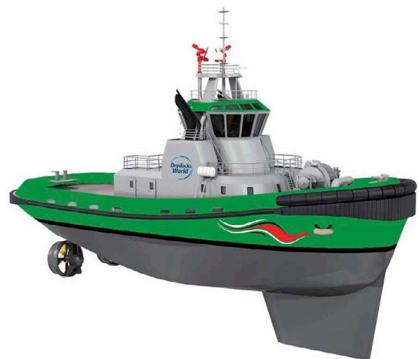
The first LNG-fuelled harbour tug in Middle East region will be designed by Wärtsilä and feature a full scope of Wärtsilä solutions (Image courtesy Wärtsilä)
