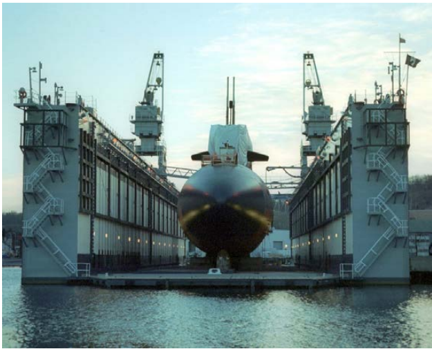
Los Angeles-class USS Dallas (SSN 700) in floating dry dock USS Shippingport (ARDM 4) in 2001 (Photo from Wikimedia Commons website)
