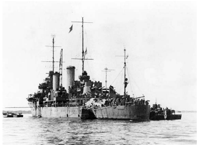
HMAS Hobart at Espirito Santo in July 1943 showing the torpedo damage to her stern (RAN Historical Collection)
