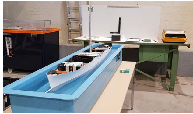
Figure 6 Set up for a model inclining experiment with an Armfield hydraulics bench at back left (Photo courtesy Warren Smith)
