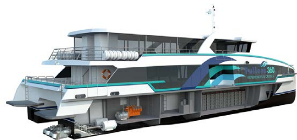
Starboard quarter cutaway view of 32 m electric ferry for Fullers360 (Image courtesy Incat Crowther)
