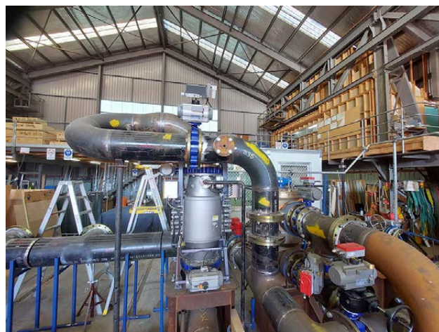
Ballast water treatment system, prefabricated in Taylor Bros' workshop (Photo courtesy Taylor Bros)
