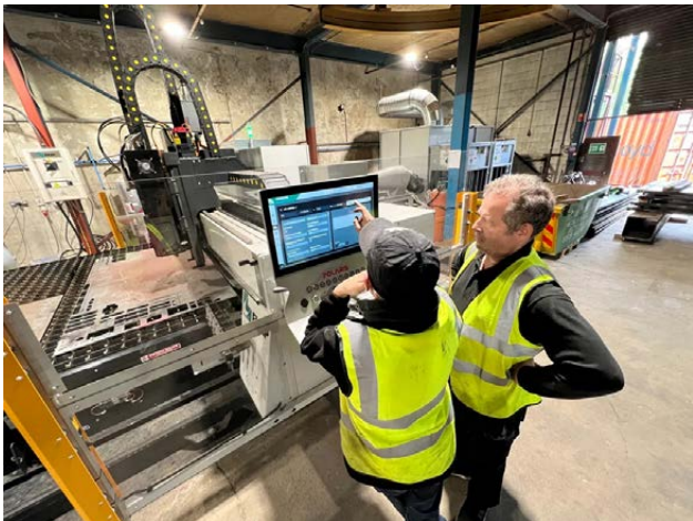
Cutting plate for the mounting cradle for Longbow's jet engines on the CNC Kronos plasma cutting machine at John W. Laycock (Photo from Longbow website)
