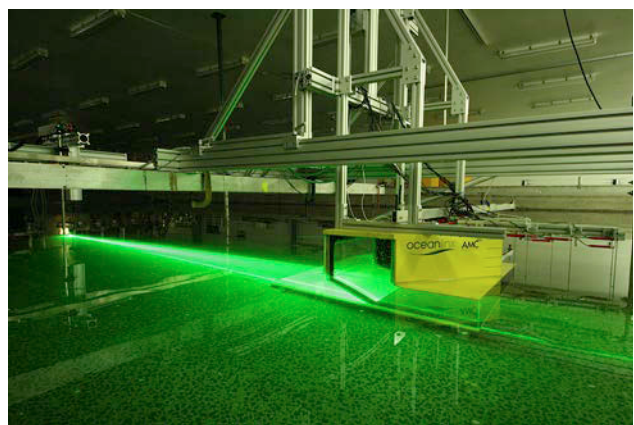
PIV experiments being conducted on a wave energy device (Photo Tom Mitchell-Ferguson, courtesy AMC)
