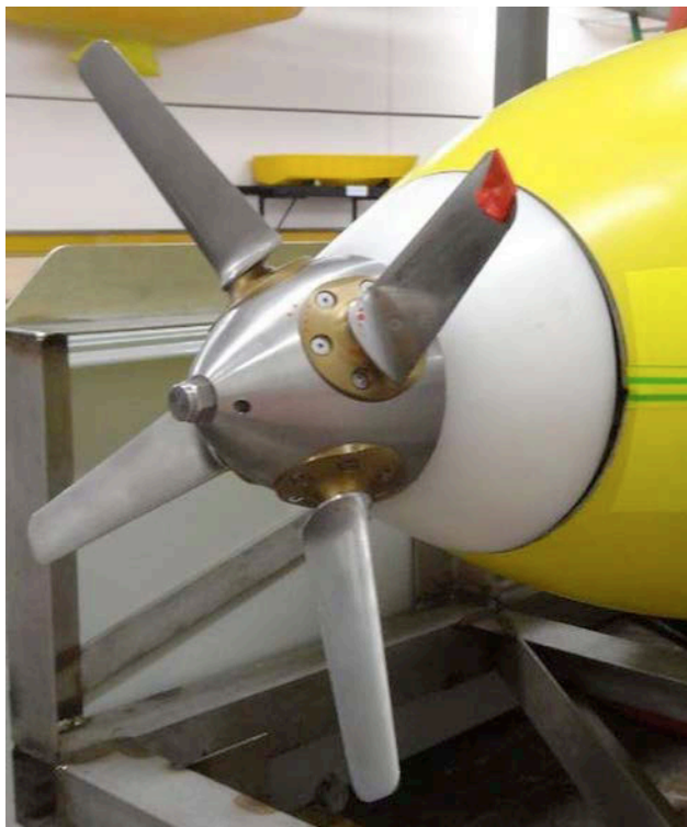
A collective and cyclic pitch propeller installed on an AUV (Photo Arno Dubois, courtesy AMC)
