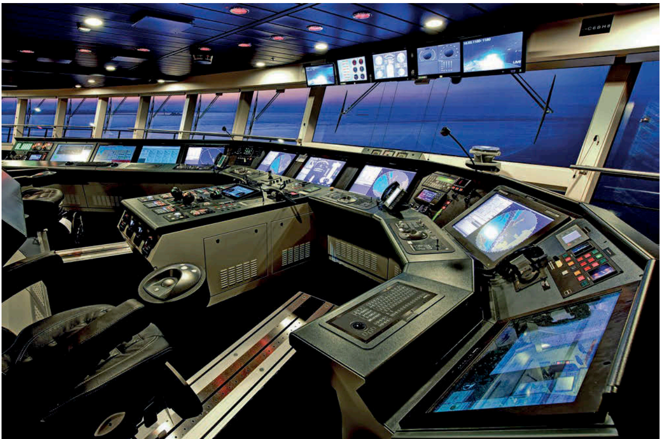
The Wärtsilä Nacos Platinum series of navigation, automation and control systems in Quantum of the Seas (Photo courtesy Wärtsilä)
