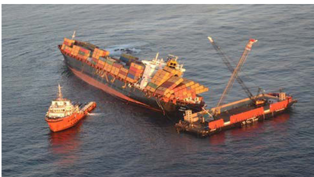
Rena with crane barge ST60 ready for cargo discharge (Photo courtesy Svitzer Salvage)
