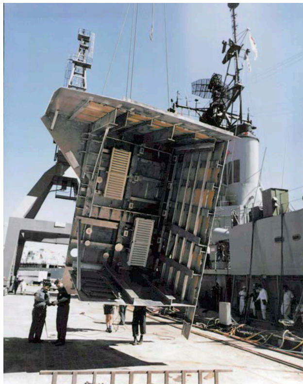
One of the CIWS magazines about to be shipped with as much outfit as possible already completed and kevlar armour fitted (RAN Photograph)
