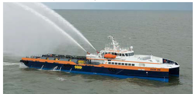
Incat Crowther-designed Seacor Lynx — A 58 m high-speed ship providing specialised services for the oil and gas industry (Photo courtesy Incat Crowther)
