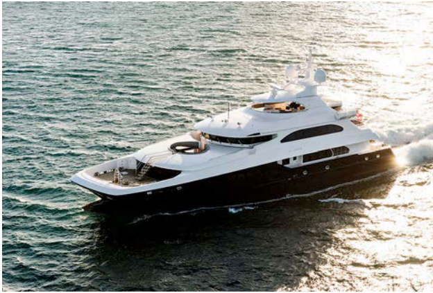
Incat Crowther-designed Zenith — a luxury 40 m aluminium-hulled motor yacht (Photo courtesy Incat Crowther)
