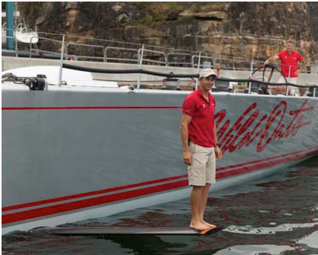
Static load on the end of a foil (Photo courtesy Wild Oats Team)
