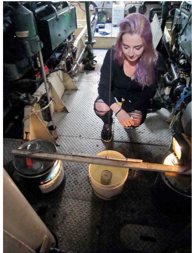
UNSW student Tamasin Welch tending the pendulum at the inclining experiment on Currawong (Photo Phil Helmore)
