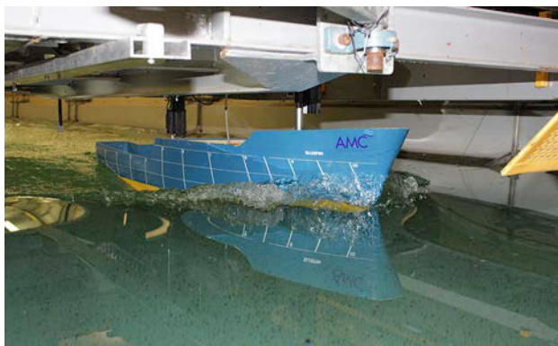
Bluefin model at a speed corresponding to 14 kn in the towing tank (Photo courtesy AMC)
