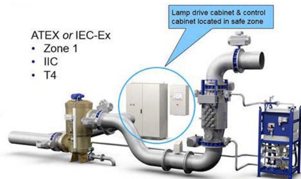
PureBallast 3.1 EX explosion-proof version (Image courtesy Alfa Laval)
