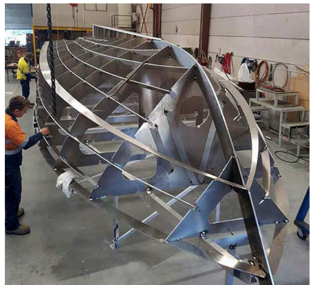
Framing of the unturned hull structure of 11.5 m fishing charter vessel (Photo courtesy John Butler Design)
