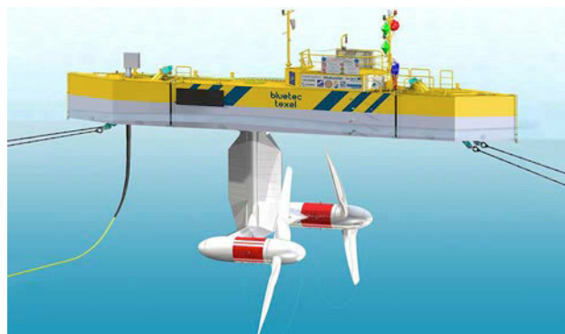
BlueTEC's tidal energy platform with Tocado T2 turbines installed giving 500 kW (Image from Damen website)
