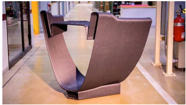
Prototype hull section of 3D printed yacht (Photo from www.3ders.org website)
