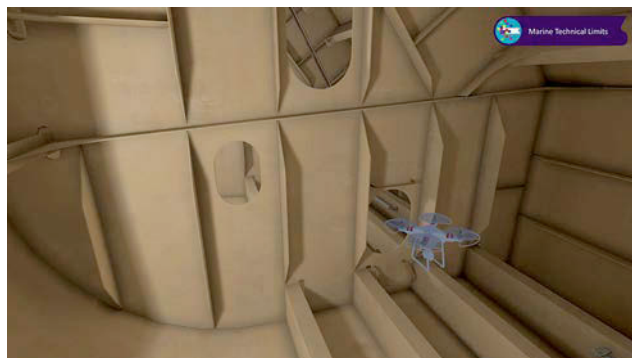
RECOMMS drone pilot training — navigating a wing ballast-tank hopper compartment (Image courtesy Marine Technical Limits)
