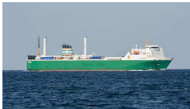
Estraden , with Flettner rotors providing supplementary power (Photo courtesy Josh Harrison)
