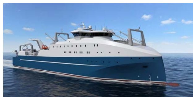
The unique bow design of the Wärtsilä-designed 121 m trawler is intended to enhance efficiency (Image courtesy Wärtsilä)
