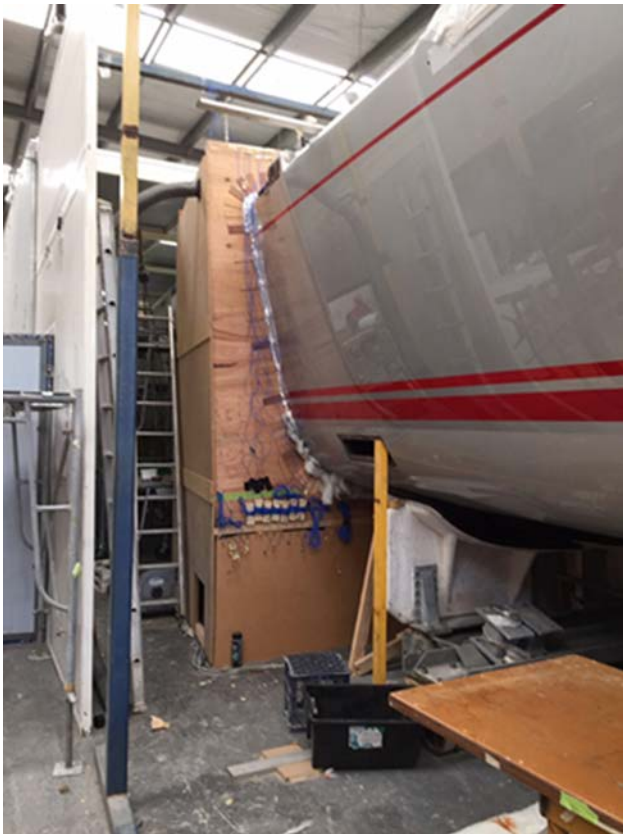
Hull join being vacuum bagged (Photo courtesy Diab Group)
