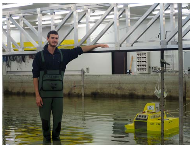
PhD candidate Jarrah Orphin conducts tests on a model wave energy converter in the model test basin at the Australian Maritime College (Photo courtesy AMC)
