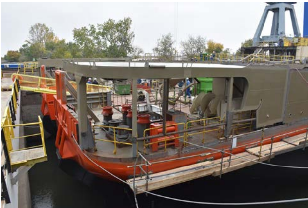
The ship's aft science deck (Deck 4) with the starboard aft mooring station in the foreground (Photo Michiel Jordaan courtesy AAD)
