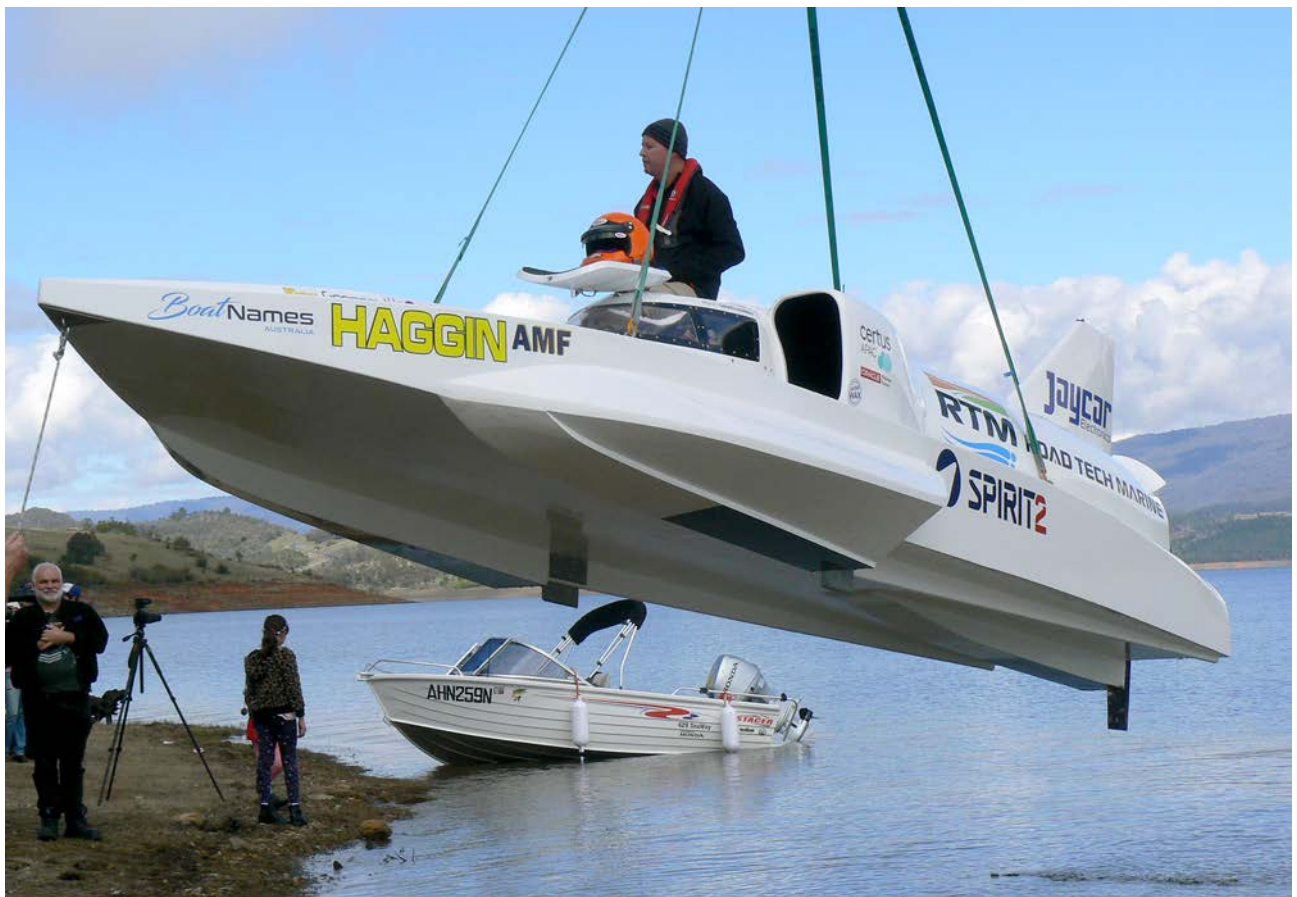
Underside of Spirit of Australia 2 being lifted from water showing fins forward (Photo Martin Grimm)
