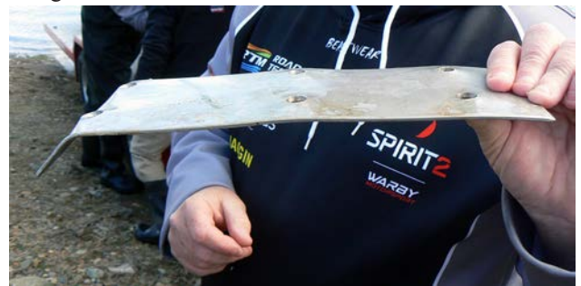
A damaged fin backing plate marks the end of trials in September (Photo Martin Grimm)
