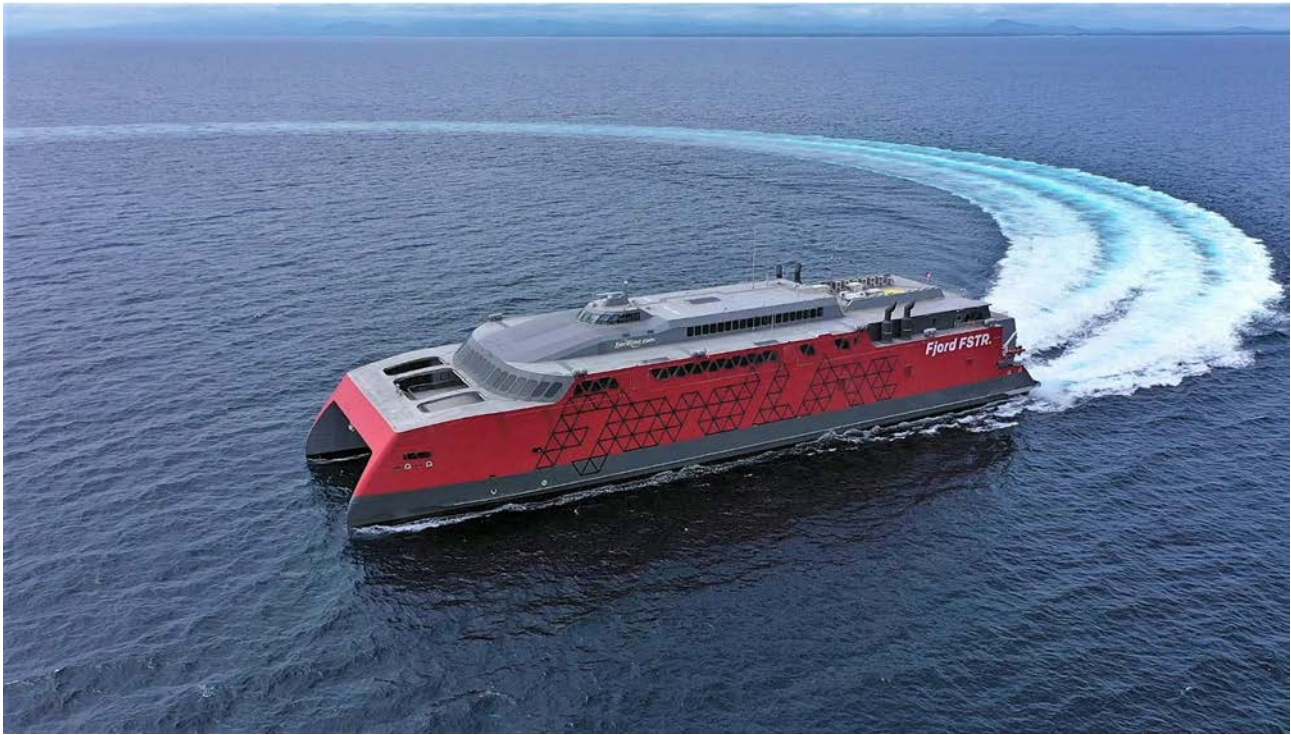
Fjord Line's FSTR , a 109 m high-speed vehicle-passenger ferry, designed by Austal Australia and constructed by Austal Philippines (Photo courtesy Austal Philippines)
