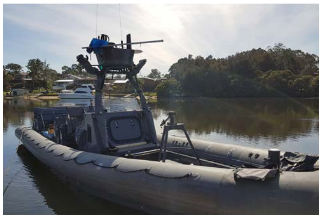
Inclining of 11 m RHIB in water (Photo courtesy John Butler Design)
