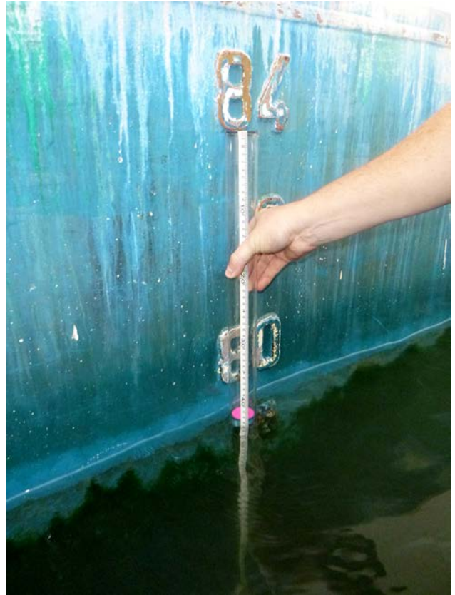
Draft measurement on Pacific Explorer (Photo courtesy John Butler Design)
