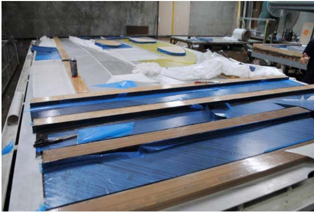
Flat structural elements being laid up (Photo courtesy McConaghy Boats)
