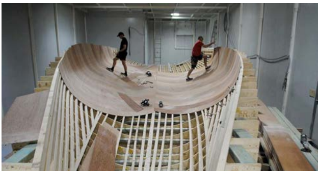
Plywood being installed (Photo courtesy McConaghy Boats)
