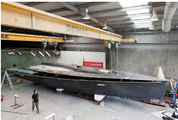
Fitting the deck (Photo courtesy McConaghy Boats)
