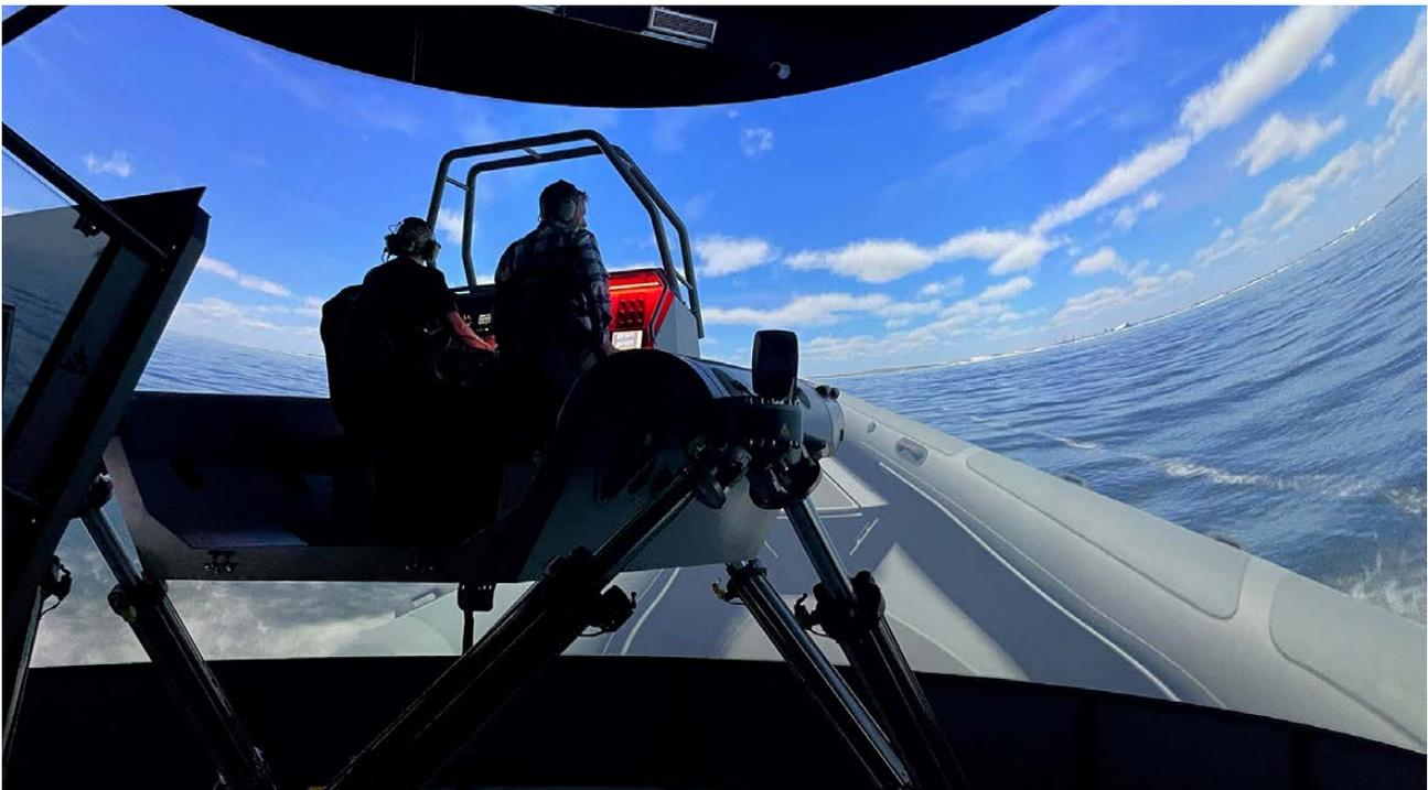
The acquisition for the RAN of new fast-craft training simulators represents an important step towards Ship-Zero simulated training capability. Acquired through Luerssen Australia, the training simulators use the latest technology to readily and safely train coxswains for challenging scenarios without having to take assets and personnel to sea
