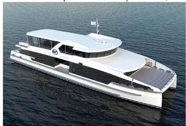
Starboard bow of 32 m hybrid fast ferry for Auckland Transport
