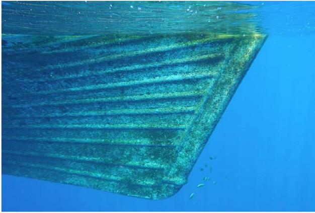
Figure 8: Seam roughness and hull fouling 10 March 2010
