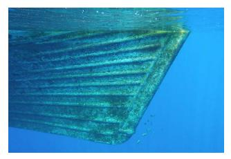
Figure 8: Seam roughness and hull fouling 10 March 2010 (Photo courtesy E. Staples)
