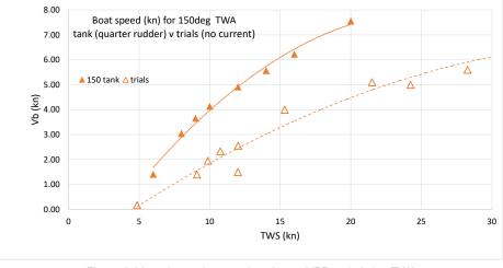
Figure 6: Vessel speed comparison log vs VPP at 150 deg TWA (Graph courtesy K. Klaka)
