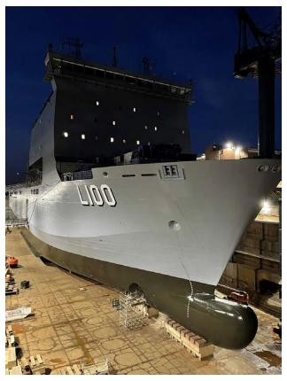
HMAS *Choules* with new antifouling applied (Photo courtesy A&P Australia)
