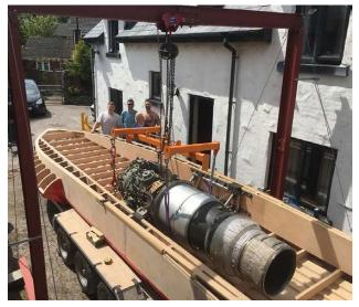
Test fitting of port jet engine in *Longbow* (Photo from Longbow website)
