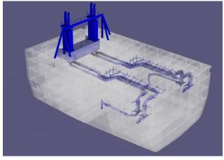
Exhaust design from engines to new exhaust stacks (midships) (Diagram courtesy A&P Australia)
