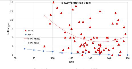
Figure 7: Leeway angle comparison log vs VPP (Graph courtesy K. Klaka)
