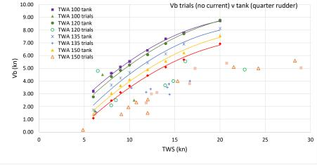
Figure 5: Comparison of vessel speeds from trials and VPP ("tank") (Graph courtesy K. Klaka)
