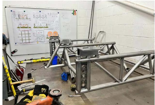
Side view of the mounting cradles for *Longbow's* jet engines
