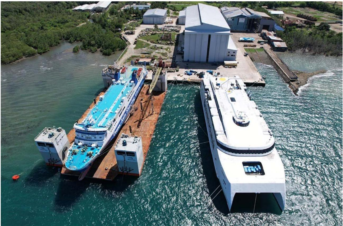
Austal Philippines recently started its first major commercial vessel servicing contract; a 110 m steel ferry for Trans Asia Shipping Lines. Utilising their own floating dock *Lewek Hercules*, the Austal team undertook repairs, cleaning and painting on the vessel
