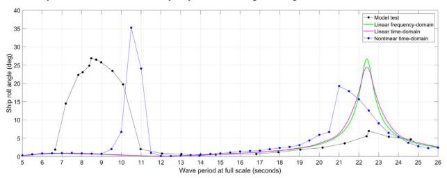
Figure 10: Comparison of measured and computed ship roll motions for the Ikeda *et al.* (2006) test case: cruise ship in regular beam seas of height 5.0 m
