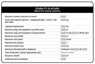
Figure 2: Example of a stability placard for a 7 m vessel (Image courtesy AMSA)
