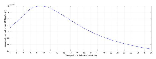
Figure 5: Wave-induced roll moment, per metre of wave amplitude, as a function of wave period
