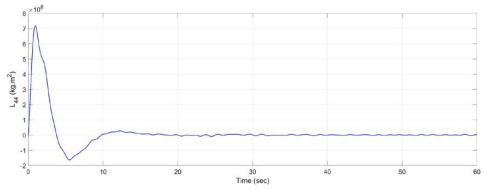
Figure 13: Roll impulse response function, as calculated using WAMIT
