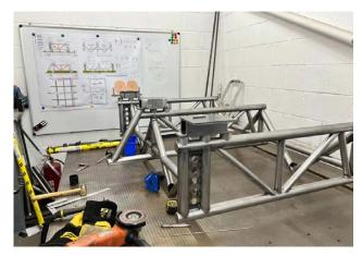
Side view of the mounting cradles for *Longbow*'s jet engines
