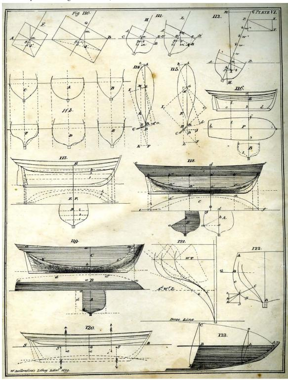
Plate VI — Figures in ilustration of the Stability of Ships and of tthe Principal Sections and Lines used in the plan
