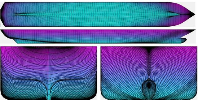
Figure 3: 14048-panel surface mesh, up to deck level, as developed with OCTOPUS 3D Mesher for hydrostatics calculations
