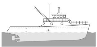
Figure 1: The proposed new freeboard mark on a 19 m fishing vessel (Image courtesy AMSA)
