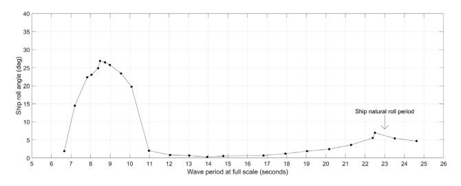
Figure 1: Measured roll angle of Fincantieri cruise-ship hull, in regular beam seas of height 5.0 m. Data from Ikeda et al. (2006, Fig. 2) and Munif et al. (2005, Fig. 3)
