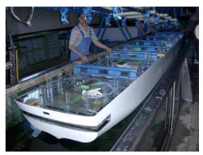
Figure 2: 1:40 scale model of Fincantieri standard cruise-ship hull, as tested at Vienna Model Basin (Photo from IMO 2004, p. 22)
