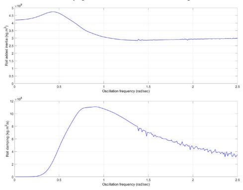
Figure 12: Roll added inertia (top) and damping (bottom), as calculated using WAMIT
