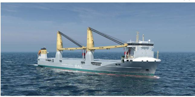
Heavy-lift vessel with methanol engines and hybrid propulsion system (Image courtesy SAL Heavy Lift)
