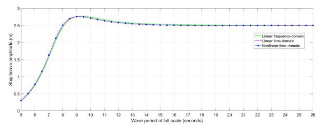
Figure 11: Computed ship heave, for the Ikeda et al. (2006) test case
