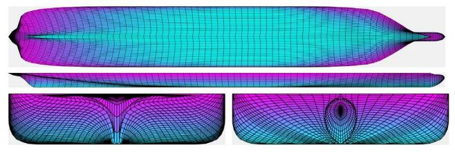
Figure 4: 3780-panel surface mesh, up to still waterline, as developed with OCTOPUS 3D Mesher for seakeeping calculations
