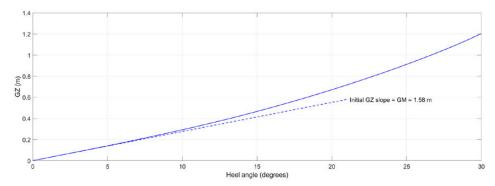
Figure 6: Calculated still-water GZ curve for the Fincantieri hull model
