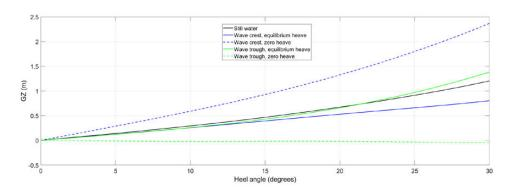
Figure 8: Righting lever curve for cruise ship in beam seas of height 5.0 m and period 8.5 seconds. Results are given for the ship in the wave crest or wave trough, and with zero heave or buoyancy equilibrium heave.
