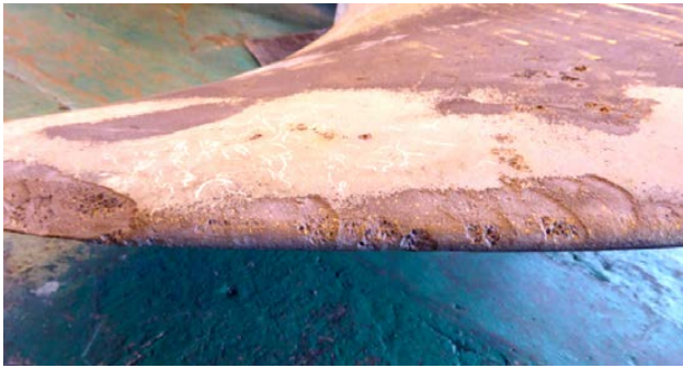
HMAS Adelaide propeller blade with tip-vortex cavitation and corrosion material removed at May 2017 dry docking after 19 months in service (Photo courtesy Defence)
