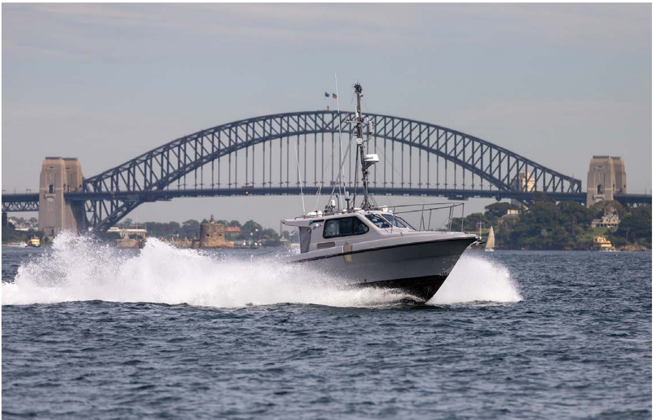
The RAN Australian Maritime Warfare Centre and Thales are testing and evaluating Steber Unmanned Surface Vehicles (USVs) for use in mine-sweeping operations. The USVs will be operating inside and outside Sydney Harbour but will be controlled remotely from a forward operating position at HMAS Watson overlooking the test area. This activity is an important step in proving the capability of the USVs before they reach full operational capability (RAN photograph)
