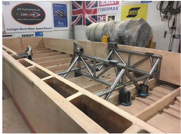
Engine- mounting cradle for Longbow ’s jet engines set up in the boat (Photo from Longbow website)
