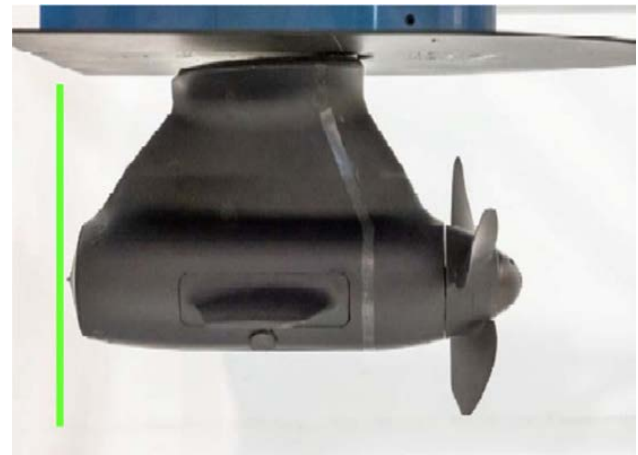
MARIN's pod model with forward propeller, and the green line showing the measurement plane of the PIV system to determine the wakefield flow into the aft propeller (Photo from MARIN Report 27507-6-DT, courtesy Defence)
