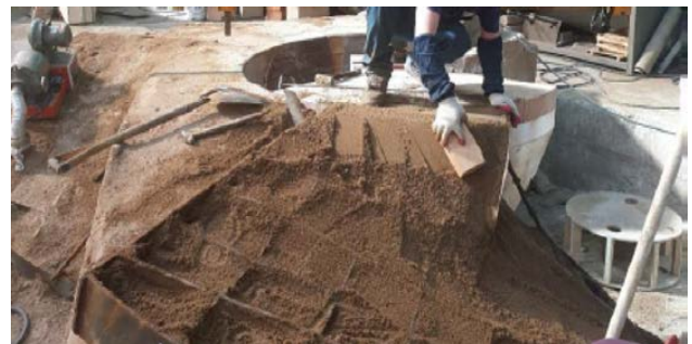
Setting up the mould for one of the new propellers (Photo courtesy Defence)
