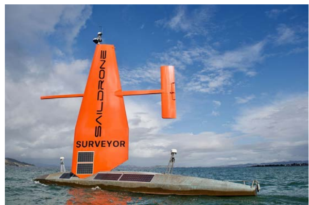
An impression of Surveyor, a 20 m long uncrewed surface vehicle designed by Saildrone (Image courtesy Saildrone)
