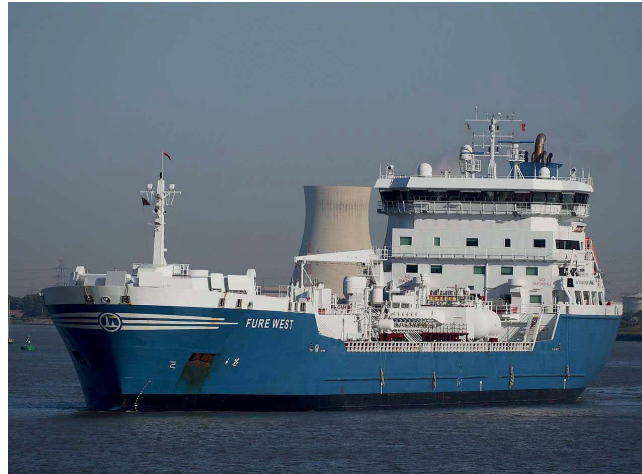
Fure West is one of first chemical tankers converted to run on LNG
