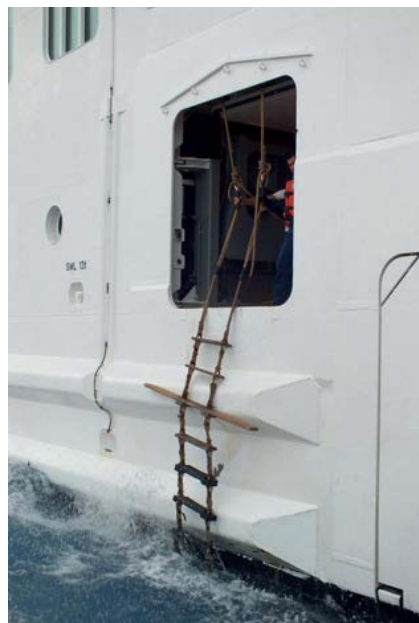
No constructional features should ever interfere with a pilot ladder
