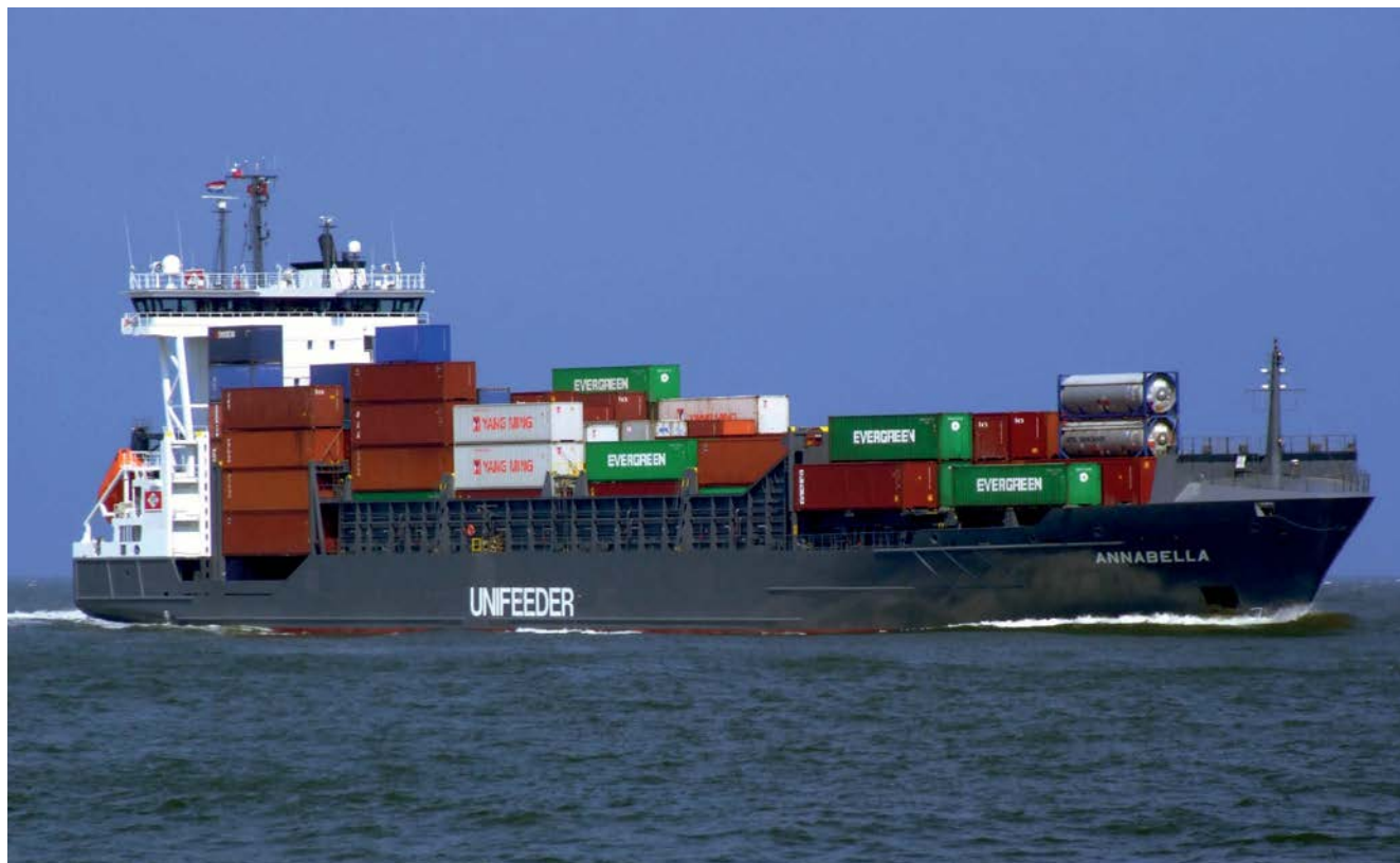
In 2007, a stack of seven 30ft cargo containers collapsed on the Annabella , raising the alarm on container stowage practices
