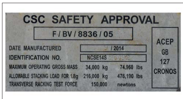
Example CSC plate, which includes information such as a container's stacking strength and racking strength
