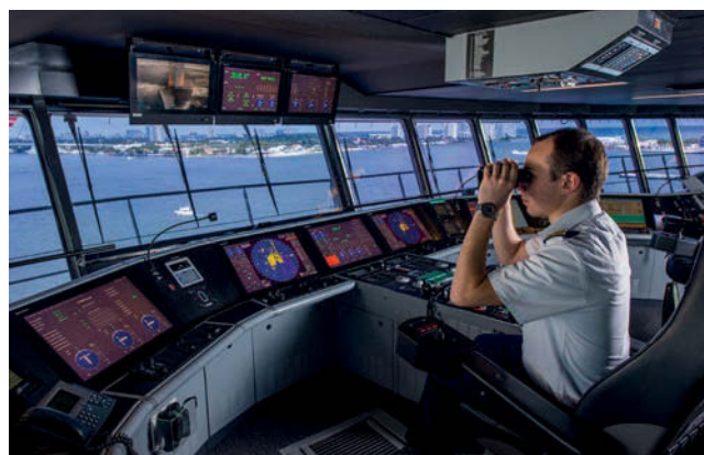
VisionMaster Net takes Sperry Marine's earlier VisionMaster FT integrated bridge solution and digitises it
