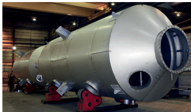
The cleaning chamber, or scrubbing tower, for Langh Tech’s scrubber system
