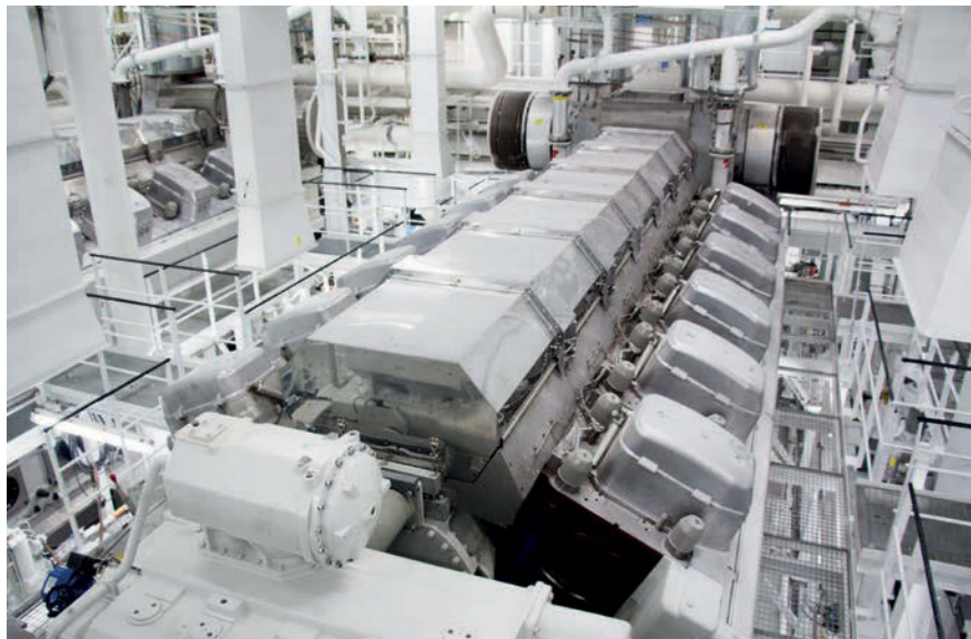
Power station at sea: looking across one of the Wärtsilä 46-series vee-form diesels in Royal Caribbean's Harmony of the Seas
