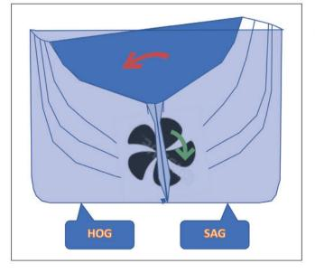
Figure 2 Sectional view from astern Torsional Deflection (Exaggerated for clarity)
