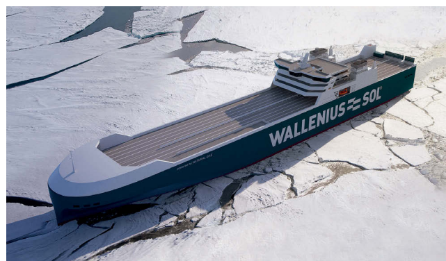
The MegaRoRo will be built to the 1A Super ice classification, allowing it to navigate in ice 100cm thick
