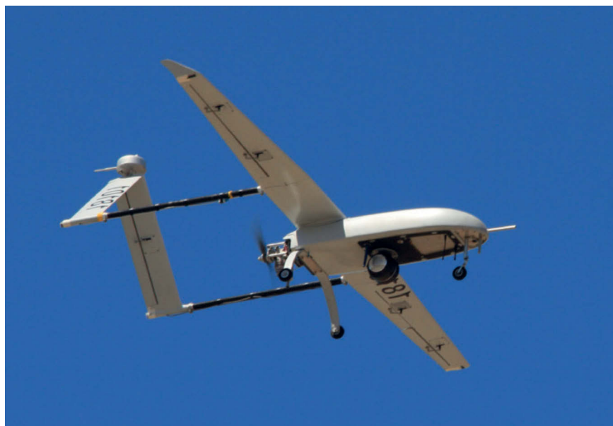
CO 2 and SO x combined sniffers installed on EMSA's RPAS can monitor emissions at sea
