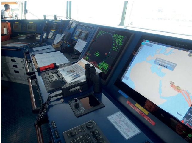
The implementation of the Electronic Chart Display and Information System (ECDIS) proved a regulatory challenge but is now mandatory on all large ships
